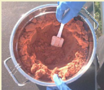
Figure 2: Stirring and drying the mixed composition over hot water.
