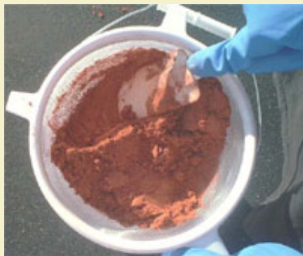
Figure 3: Screening the dried composition.
