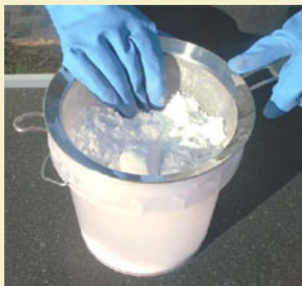
Figure 1: Screening potassium perchlorate individually into a plastic container.
