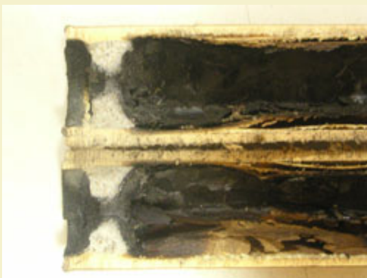
Figure 2: The same rocket with a curved inner plug surface suffered no signs of burn-through.
