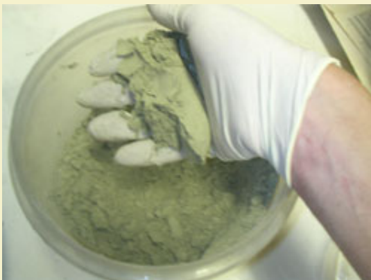
Figure 5: Working the wax solution into the clay.
