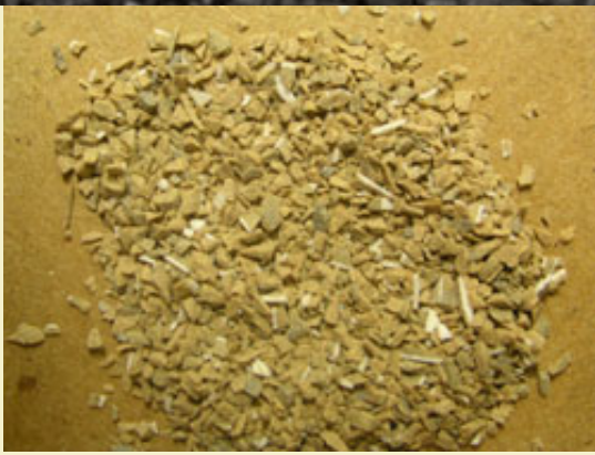
Figure 8: Close-up of 25-40 mesh tile fragments showing the sharp edges.
