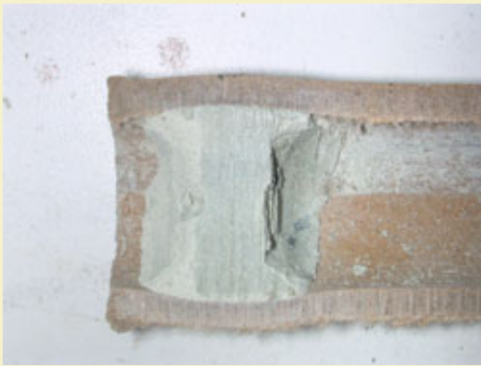
Figure 9: Weaker tubes will allow the clay plug to expand beyond the inside diameter by bulging out the case wall, which locks in the plug and makes it much more difficult to blow out.
