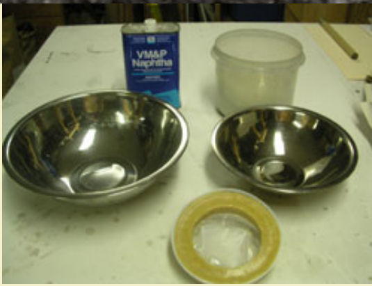
Figure 3: Supplies required for adding wax moisture resistance to bentonite clay.
