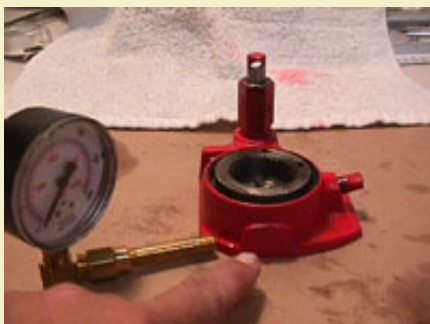
Figure 5: Using gauge assembly to mark center of side hole.
