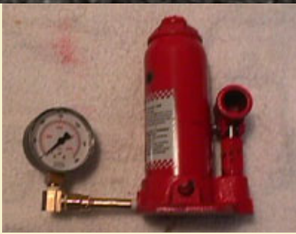
Figure 8: Reassembled jack with new gauge.
