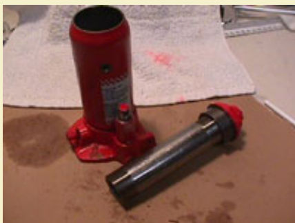
Figure 2: Removal of the piston.
