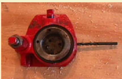
Figure 6: Checking the depth of the side hole.
