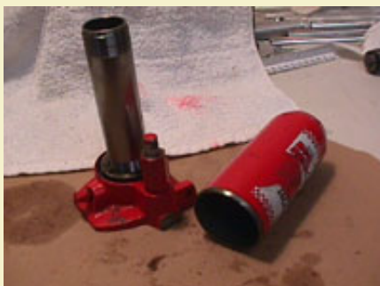
Figure 3: Removing the outer case.
