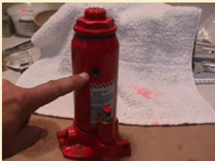
Figure 1: Remove the oil plug and drain all fluid.
