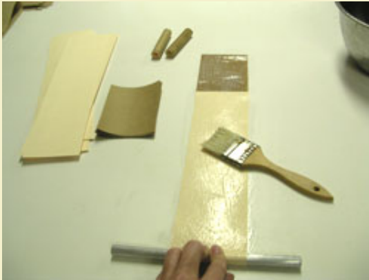
Figure 4: Rolling the rocket engine tubes.
