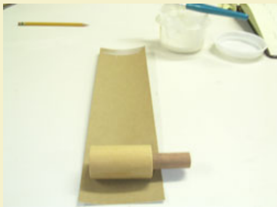
Figure 10: Rolling the header on a special former.
