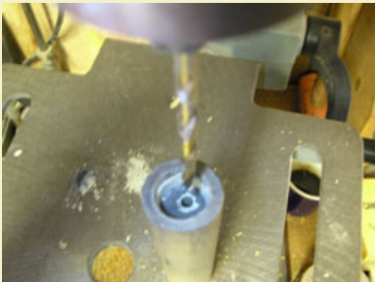
Figure 9: 1/8" passfire hole drilled through end plug.
