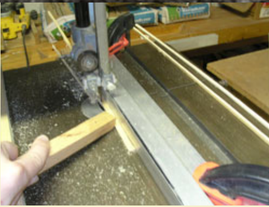
Figure 19: Using a push-stick to safely feed the tiny strip into the blade.
