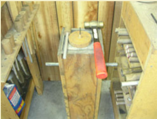
Figure 5: A cement filled ramming block and brass hammer for loading the engines.
