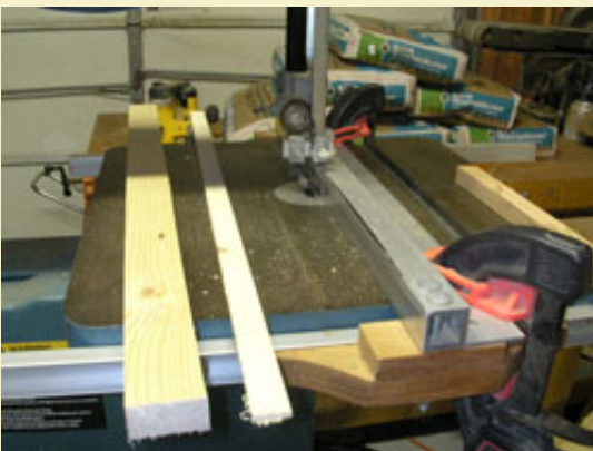
Figure 18: The slice is laid flat and is ripped into three sticks.
