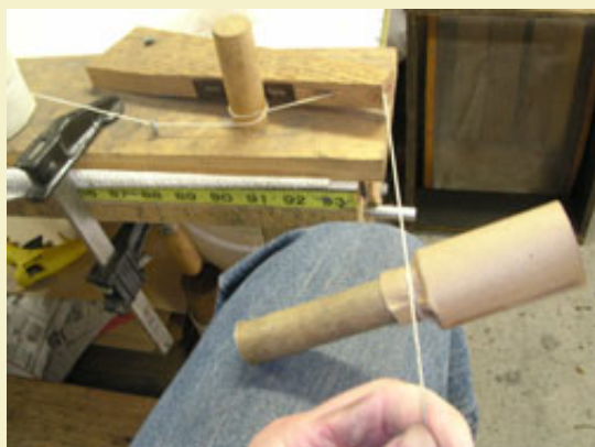
Figure 12: Using a spiking horse to apply a tight half hitch over the glued header collar.
