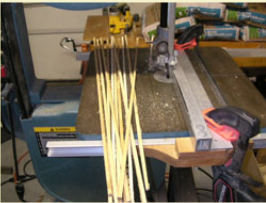
Figure 20: Dozens of rocket sticks cut from a small stick of wood.
