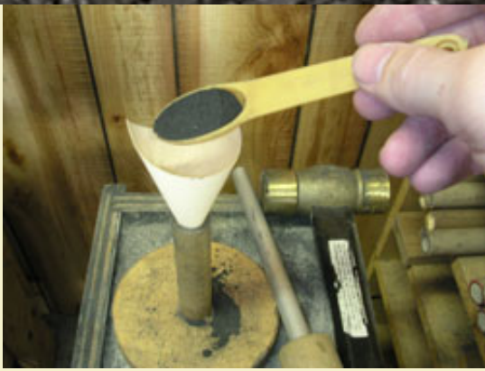
Figure 7: Adding a 1 TSP (5 ml) increment of BP fuel.
