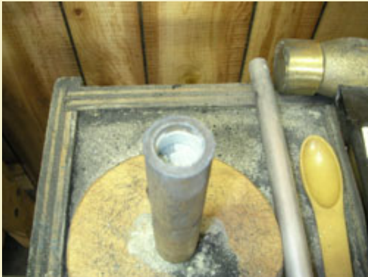
Figure 8: The clay end plug rammed in place.
