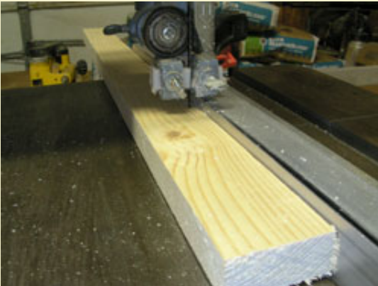
Figure 17: Making a slice off the edge of a knot-free 3/4" thick board.
