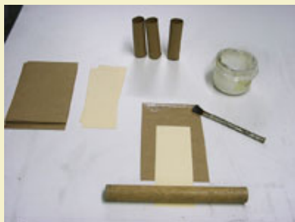
Figure 1: Paper cut and ready to roll saettine cases.
