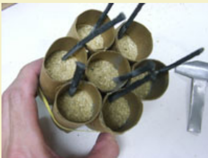
Figure 4: Packing in the sawdust for delay.
