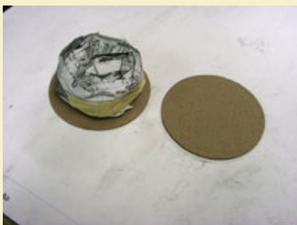
Figure 8: Piston made with wadding between two solid disks.
