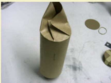
Figure 7: Pleating the bottom of the mine bag.
