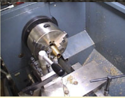
Figure 4: Turning a taper on the brass sleeve allows easier insertion into dense comp.
