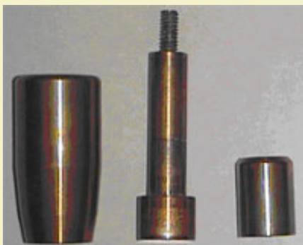
Figure 2: Components of the pump include sleeve, piston and pounding nub.
