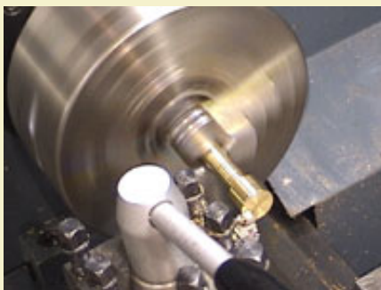
Figure 3: Turning the piston from a piece of \frac{3}{4} " brass rod.
