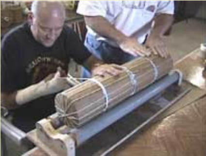
Figure 5: Using a roller to spike between the breaks of a large shell.
