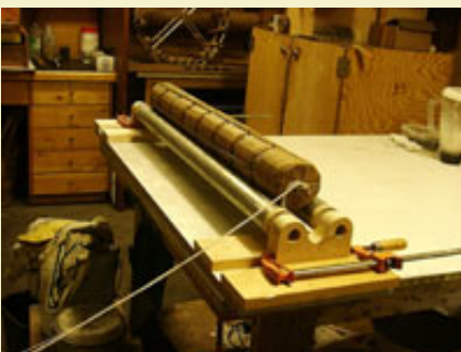
Figure 7: Roller adjusted to narrow spacing to handle a long multi-break 4" shell.
