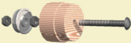
Figure 1: Details of the roller plug assembly.
