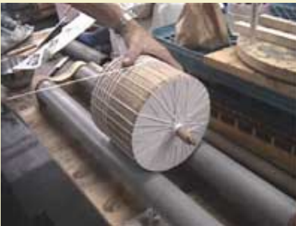
Figure 6: Using a roller to apply horizontal spiking on a bottom shot.
