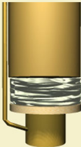
Figure 8: Shell, paper wadding, wooden disk and lift charge.
