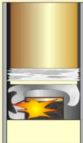
Figure 11: Case bursts, sending pressure impulse that forces wood disk upward.
