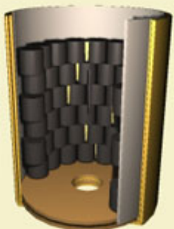
Figure 2: Comets held tightly in rings with wooden wedges.
