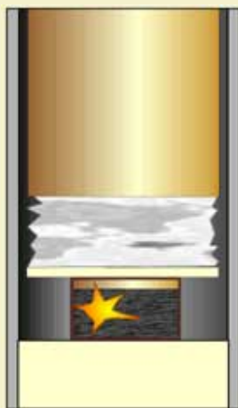
Figure 10: Pressure builds in lift charge case.
