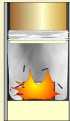
Figure 12: Wood disk compresses sabot, trapping all lift gas and sending shell
