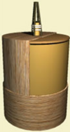
Figure 4: Solid spiking with single ply jute twine.
