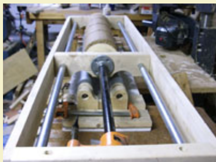
Figure 8: End view of press frame sitting over the roller.
