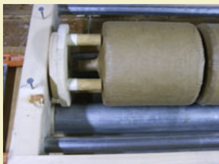
Figure 7: Fingers are long enough to allow room for spolette.
