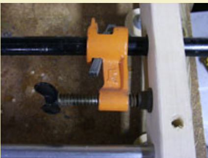
Figure 5: The reversible pipe clamp provides the force.
