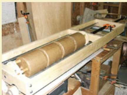
Figure 6: Four 6" shells being compressed together.
