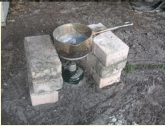
Figure 19: Using a Coleman propane burner to melt 10 lbs of lead out doors.
