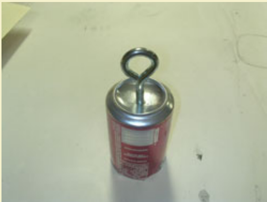
Figure 18: The bottom of the soda can is fitted with an eyelet so that it can be suspended from bungee cords or springs.
