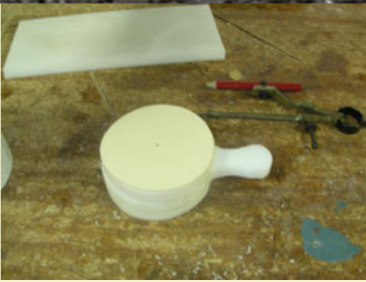
Figure 22: The three disks are fastened together using double sided carpet tape so the pieces will not slide during drilling.
