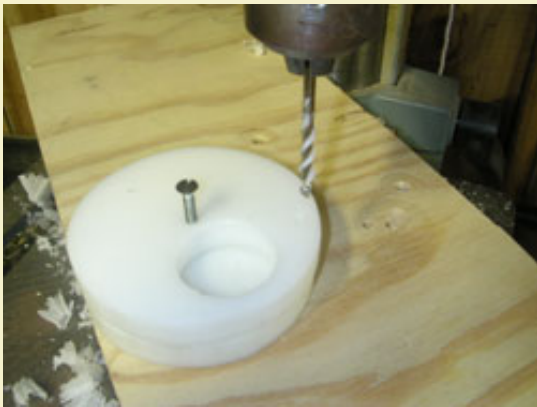
Figure 26: The top plate is placed over the bottom plate and used as a template when drilling the brass pin hole so that the two pieces will be correctly aligned.
