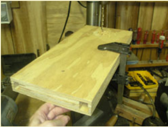
Figure 2: Clamping the opposing sides of the base box together when drilling the 5/16" tie-rod holes.
