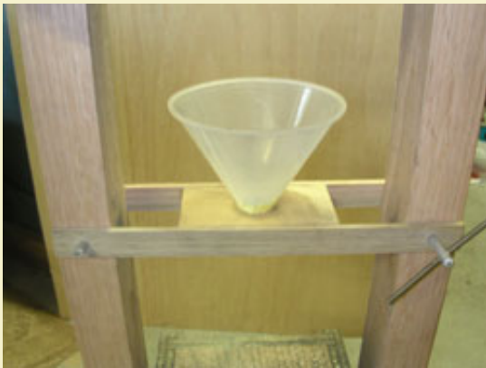
Figure 16: The hinged funnel plate set in place with the right-hand lock pin.
