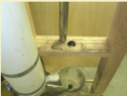
Figure 36: Resting the rammer on the center support while loading driver tubes.
