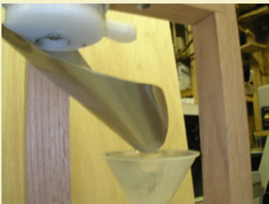
Figure 33: Powder chute is pinned between the powder dispenser and the frame.
