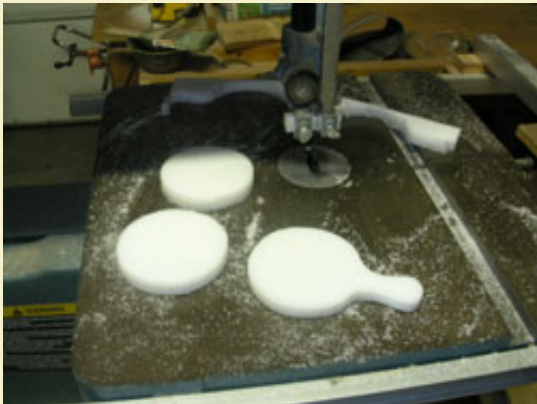
Figure 21: Cutting the 3" diameter disk set out of the chopping block material, which will be used to make the powder dispenser.
