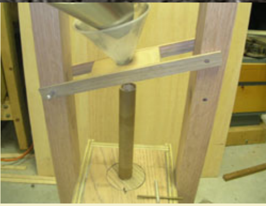
Figure 34: A tube being loaded into the completed driver rammer.
