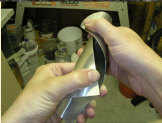
Figure 31: Twisting a sheet of aluminum flashing to produce the powder chute.
