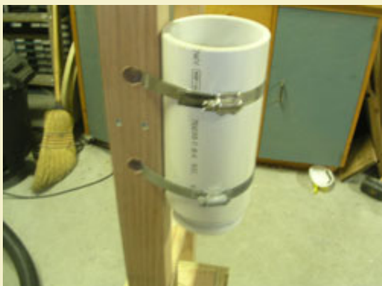
Figure 29: The powder dispenser unit is attached to the left side of the frame using pipe clamps running through holes drilled in the frame.
