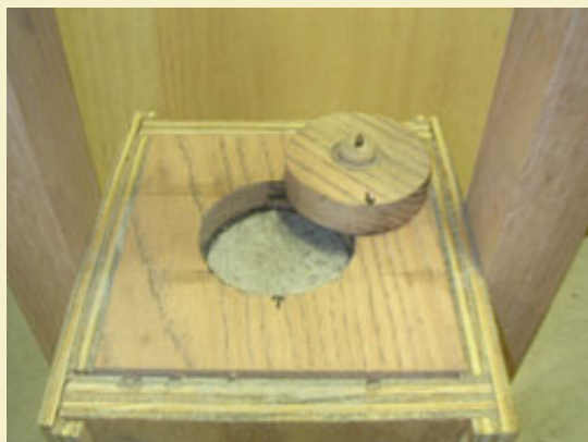
Figure 13: A hole is cut at the rammer center point on the base top plate so that interchangeable ramming bases can be used.
