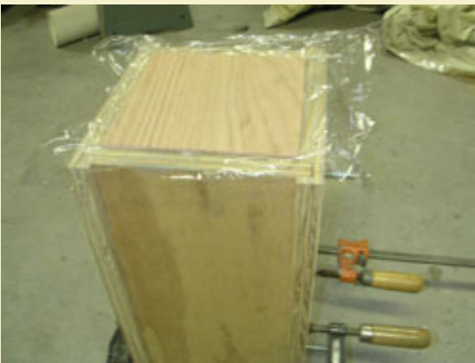
Figure 7: A sheet of thin plastic food wrap is placed over the wet cement, then the top block is tapped into place using a rubber mallet.
