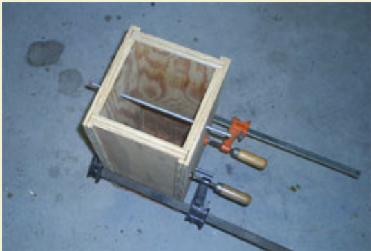
Figure 4: The two tie rods are run through the side holes prior to filling the box.
