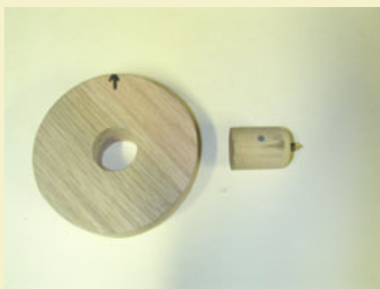
Figure 14: Components of a 3/4" ramming base with center marker for making drivers. Note small nail holding the brass center pin in place.
