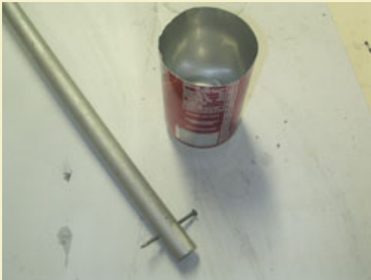
Figure 17: A hole is drilled through the top of the ramming rod so that it accepts a nail. The top of a soda can is cut off so it can be used as the form for casting the top weight.
