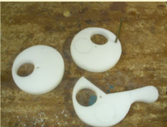
Figure 24: The completed plate set, with the special slice removed from the inner rotating plate.
