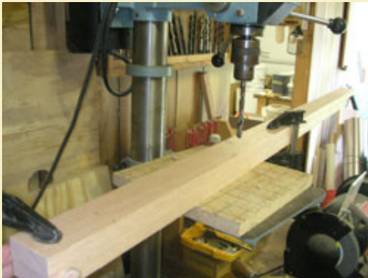
Figure 8: Clamping the 54" long and 36" long frame pairs together when drilling the tie-rod holes.
