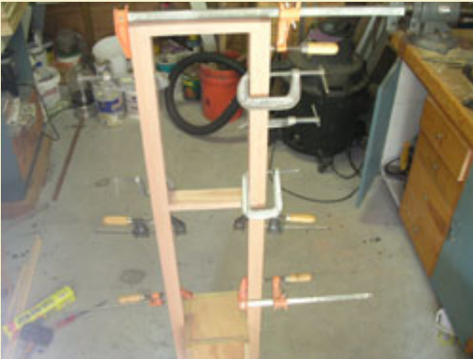
Figure 11: The 16-1/2" segments are now glued and clamped into place, while the unglued cross members are laid in place for spacing purposes.
