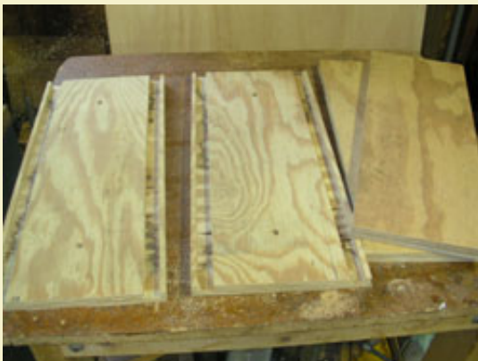
Figure 1: Pieces cut for the base box that will hold the concrete.
