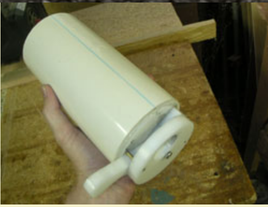
Figure 28: The powder increment device is hot glued into the bottom of a 3" I.D. PVC pipe, which will be the powder store for granulated composition during use.
