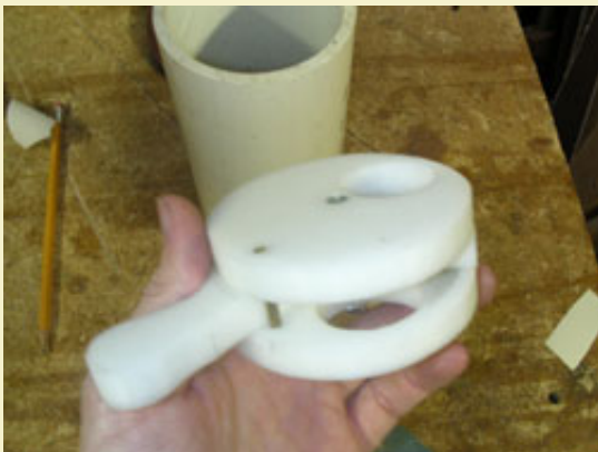
Figure 27: The completed powder increment device showing the entry hole on top and the exit hole on the bottom.
