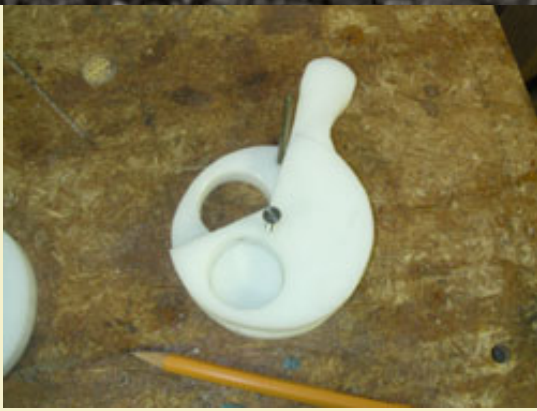
Figure 25: The brass stop pin serves as a rotation limit as well as a means to keep the bottom plate aligned with the top plate while the inner plate rotates.
