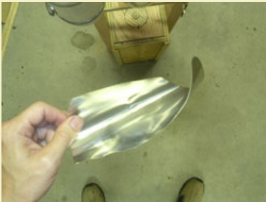
Figure 32: The completed powder chute that will carry powder from the dispenser to the funnel.
