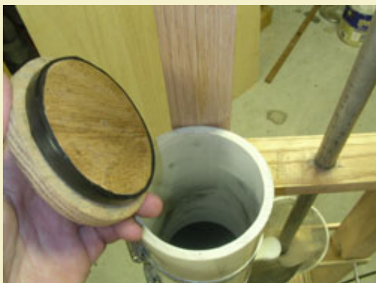
Figure 30: A wooden lid is made to close off the top of the powder store, since standard PVC caps can not be used.
