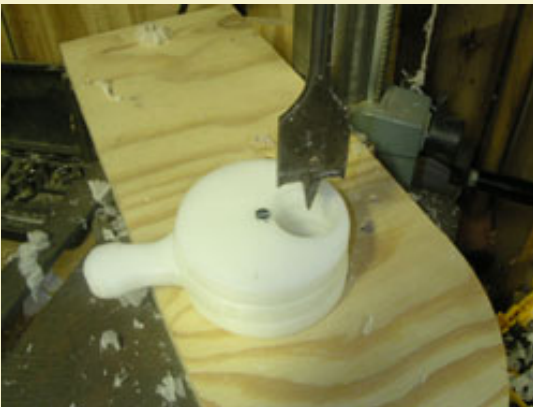
Figure 23: After the center hole is drilled, the machine screw is put in place before drilling the 1-1/8" diameter powder increment hole through all three plates.
