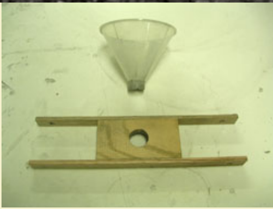
Figure 15: The funnel plate is made using the shorter cross member in Figure 12 as a drill guide. Two 1/4" wide support bars are glued to each edge.
