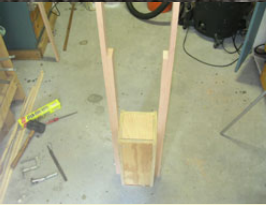
Figure 10: The tie rods are used to clamp down the side members using a washer and nut on each one.
