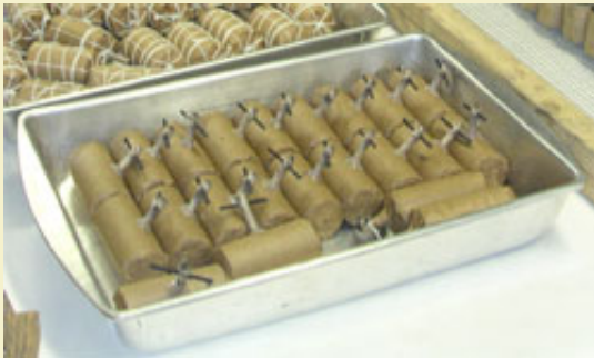
Figure 8: A tray of 20 side fused reports ready for loading.
