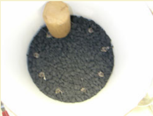
Figure 4: Loading the second ring of insert shells after filling in with rough powder.
