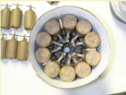
Figure 9: Third compartment is loaded with two rings of 10 reports.
