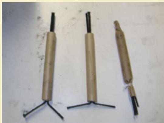
Figure 1: Two pass-through spolettes and one charged spolette.
