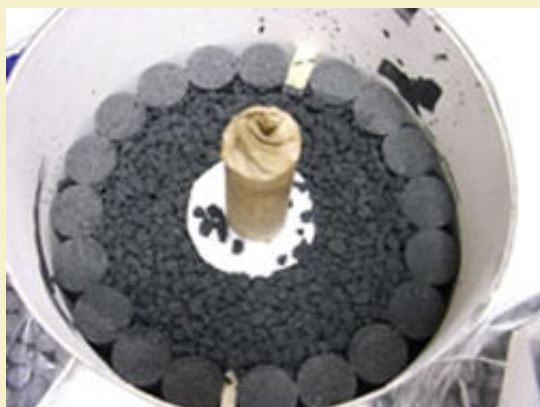
Figure 2: The top compartment, a standard Maltese color break with a 3.5sec spolette.
