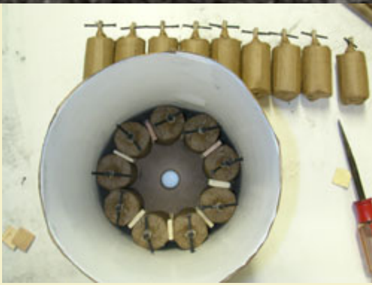
Figure 3: Loading the first ring of insert shells in the second compartment.
