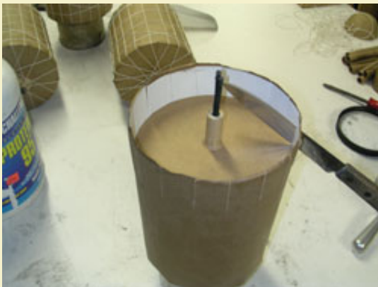
Figure 10: All three cans are closed using the Maltese method.
