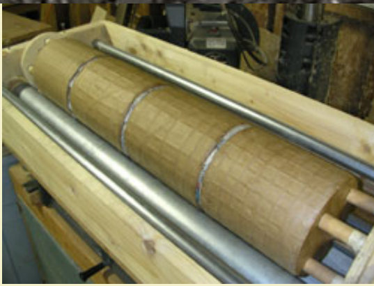
Figure 14: Newspaper rammed in place while press aligns shells tightly together.
