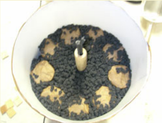
Figure 7: Rough powder is filled around the spolette and all other empty spaces to finish off the second compartment.
