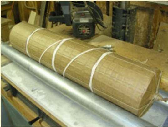
Figure 15: Eight verticals hold shells together, with cotton twine wrapped tightly between breaks to tighten vertical twine.
