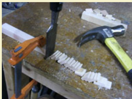
Figure 18: Cutting wooden wedges using a hammer and chisel.
