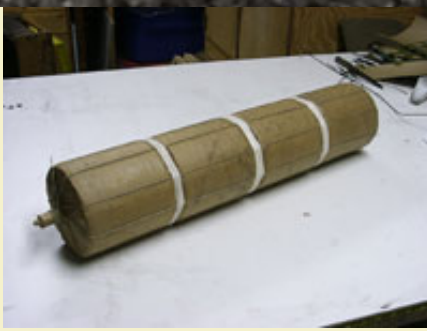
Figure 39 Stringing between the breaks with cotton twine.
