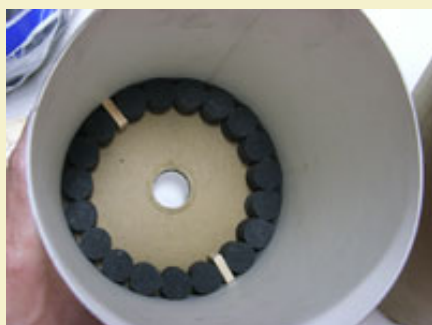
Figure 19: Wedges used to lock each row of stars tightly in place.
