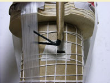
Figure 48: Bending the black match over before inserting leader into lift can.
