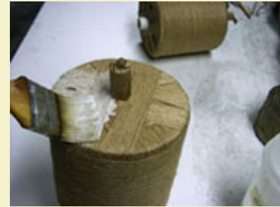
Step 6: Applying glue/paste solution to top and bottom of spiked shell.
