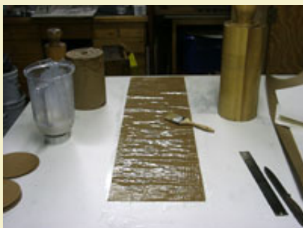
Figure 2: Paste is painted onto one side of 9.5" x 36" 60lb recycled kraft. Grain direction does not matter.
