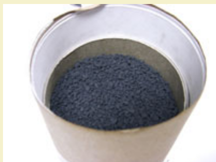
Figure 43: Can filled with 250 grams of 1/8" rough powder.
