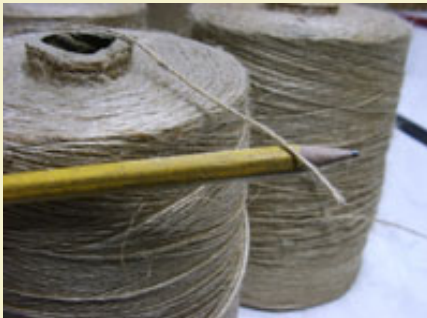
Figure 26: A special single ply jute twine used to spike color breaks.
