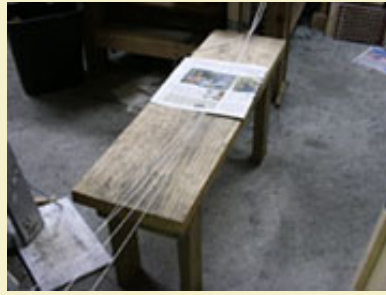
Step 2: Twine runs between two sheets of newspaper, which the worker sits on, then loops through an eyelet in front.
