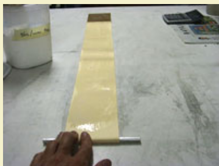
Figure 8: Strips are laid end to end and painted with a 50/50 mixture of white glue and water.
