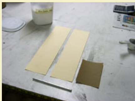
Figure 7: Two 14.5" strips of file folder paper and a piece of 30lb kraft for rolling spolettes.
