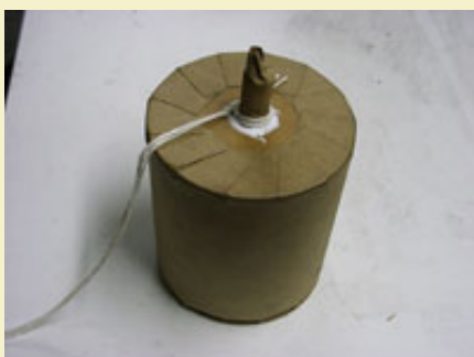
Figure 16: A second solid disk is placed on the bottom, then glue is applied around the spolette prior to spiking.
