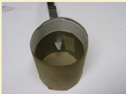
Figure 42: Punching fuse hole in lift cup.
