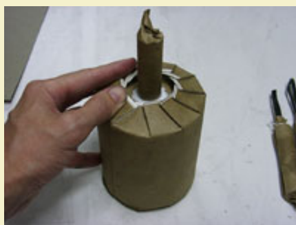
Figure 13: Folding tabs down over disk.
