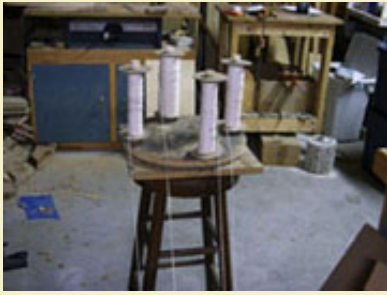
Step 1: Four spools or cones of cotton twine are placed behind the worker.
