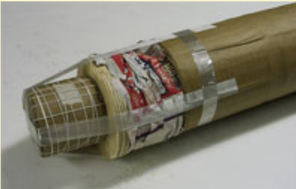
Figure 47: Fiber tape holding lift components in position.
