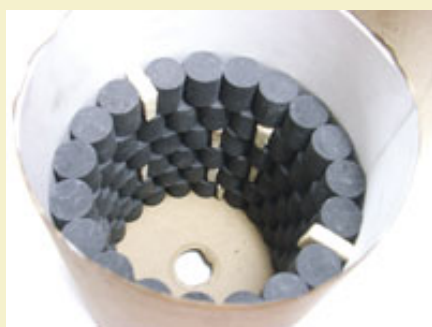
Figure 20: Six rows of nineteen stars per break.
