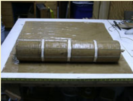
Figure 40 Pasting in the shell.
