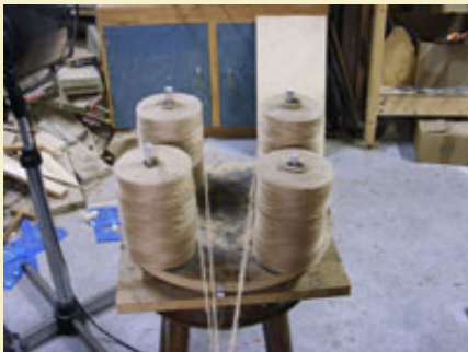
Figure 27: Four spools are used to apply four strands at a time.
