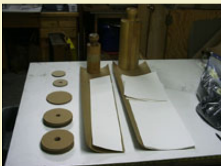
Figure 1: Punched disks, 60lb kraft strips and poster board strips for making four 6" cans and one 4" can.
