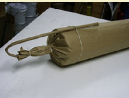
Figure 51: Finish wrap at top of shell.
