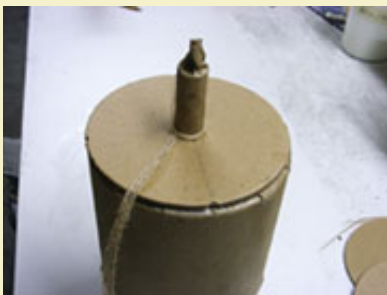
Figure 28: Four strands are passed through spiking eyelet and tied off to spolette.
