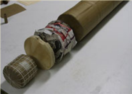
Figure 46: Lift can, plywood disk and paper wadding in assembly order.
