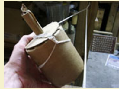
Step 3: Spiking begins by tying off around the shell itself, rather than the spolette.
