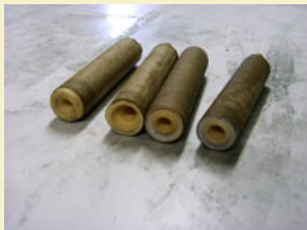
Figure 9: Finished spolette tubes ready for drying.
