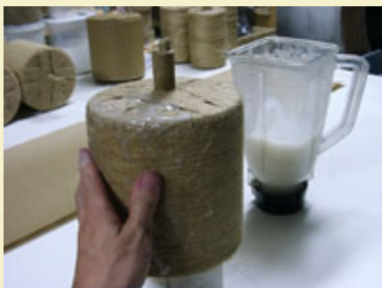
Figure 29: Coating the twine with paste.
