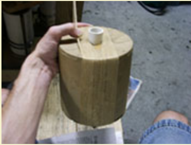
Step 1: Vertically wrap solid, wide bands of twine on both sides of center.
