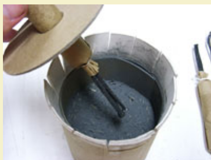
Figure 12: 300 grams of flash mixed with rice hulls.
