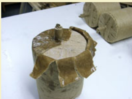
Figure 31 Pleating over the ends.
