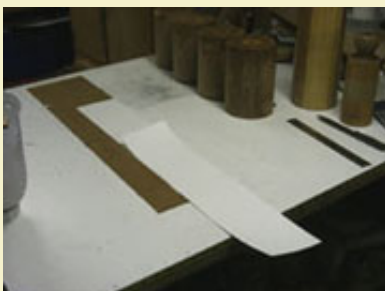
Figure 5: The salute can gets four turns of poster board.
