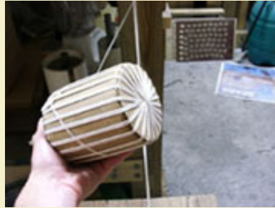
Step 5: When the verticals are complete, the twine is run down the side to the bottom and spiked in the other direction. This horizontal spiking is also spaced at 1/4".
