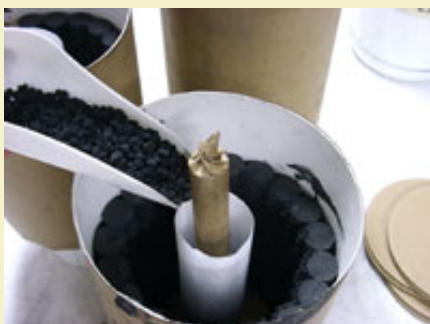
Figure 22: Filling tissue paper burst bag with 1/4" rough powder while spolette is held in place.
