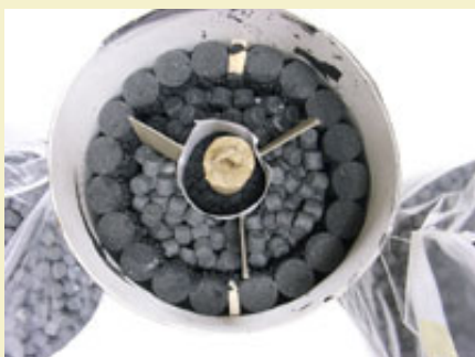
Figure 23: Temporary chipboard dividers used to section off three color compartments.
