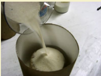
Figure 14: The 4" salute is inverted into the 6" can with the 5/8" hole, then filled around with sand..
