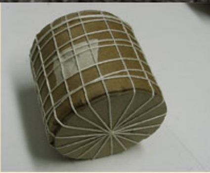
Figure 45: Finished lift can with tapped over fuse hole.
