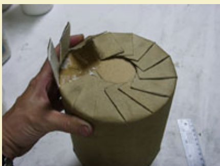
Figure 15: A solid disk is placed over the sand, then tabs are cut and folded.
