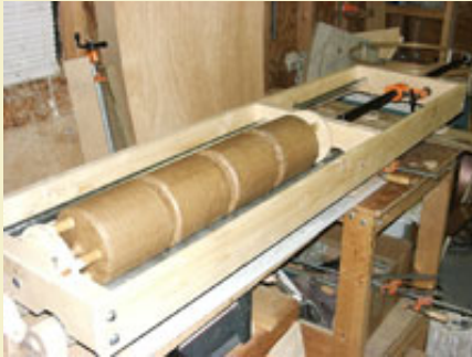
Figure 36: Shell press setup over shell roller.
