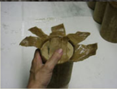
Figure 6: A single solid disk is pleated over using only the kraft paper.
