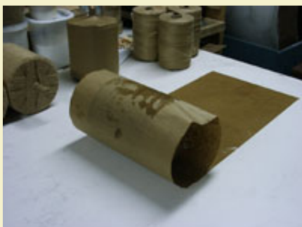
Figure 30: Rolling on two turns of pasted 30lb kraft.
