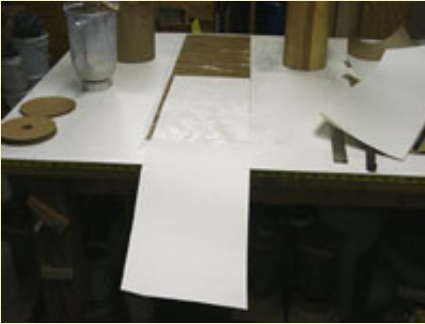
Figure 4: Poster board overhangs the kraft half its length. Paste is applied to the poster board only where it overlaps the kraft.
