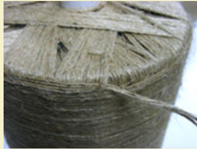
Step 5: Slip last horizontal wrap under a few plies of twine from atop the shell and glue the loose end.
