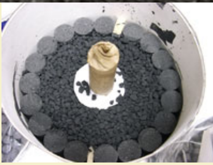
Figure 24: Rough powder used to fill in level with top of comet rings.
