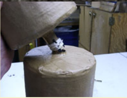
Figure 35 Stacking the breaks upside down.
