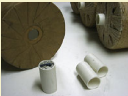
Figure 21: Plugging bottom holes with PVC plugs.
