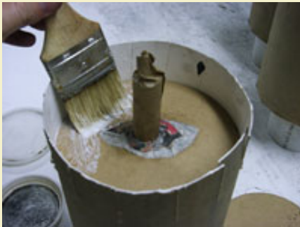
Figure 25: Pasted newspaper sealed around spolette. Glue and fold tabs as shown previously.
