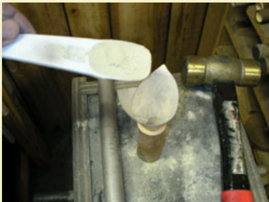
Figure 7: Loading 1/2 tablespoon of clay for the end plug.
