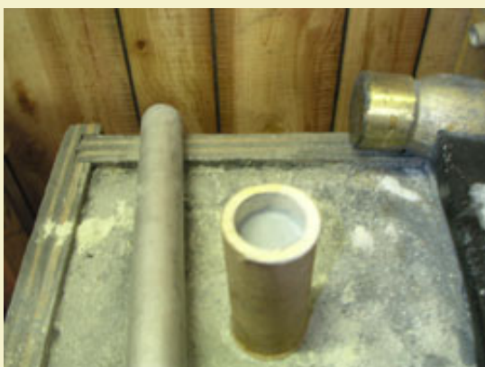
Figure 11: Stopping point for smoke composition before loading clay plug.
