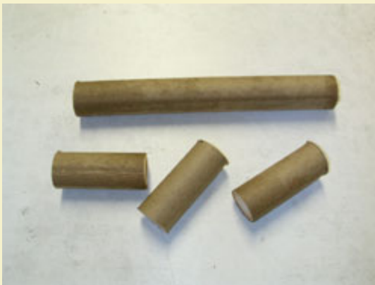
Figure 5: Cutting smaller tubes from a long one.
