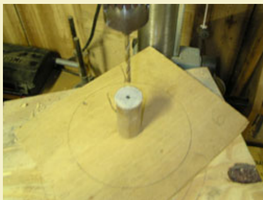
Figure 12: Drilling the 1/8" vent hole.
