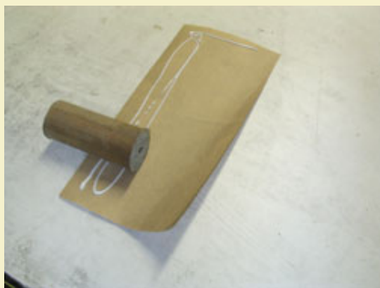
Figure 13: Applying the nosing paper.
