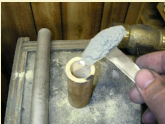
Figure 10: Loading a scoop of smoke composition.
