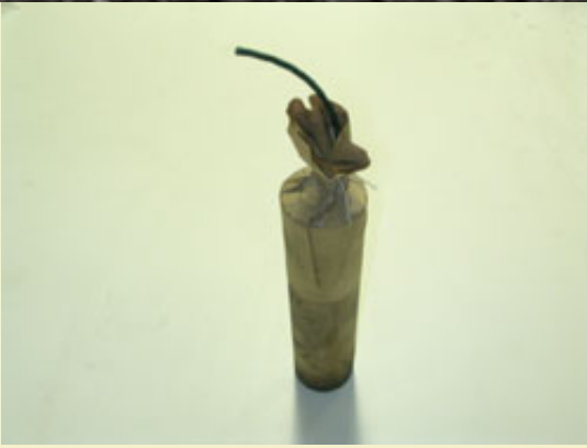
Figure 12: The finished gerb.
