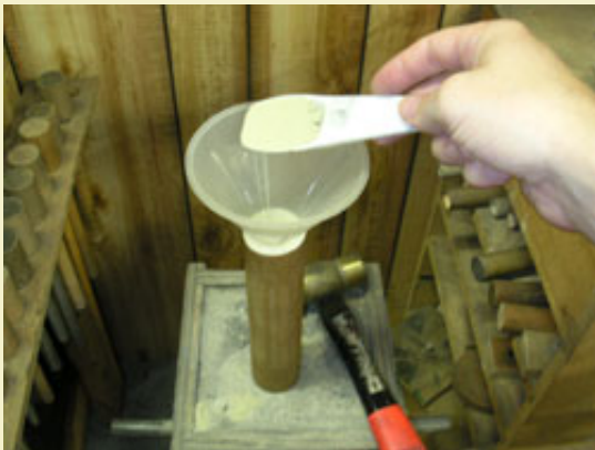
Figure 8: Making the clay plug.
