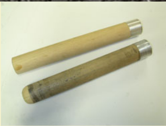
Figure 6: Wooden dowel rods used as rammers.
