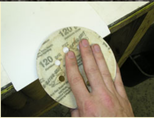
Figure 3: Sanding the inside edge to a taper.
