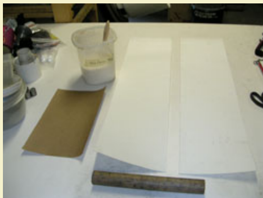
Figure 2: Rolling the casing from poster board.
