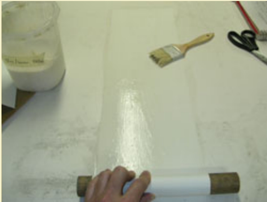
Figure 4: Coating one side with 50/50 white glue/water.
