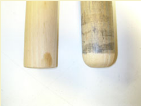
Figure 7: The plug forming rammer has a rounded tip.
