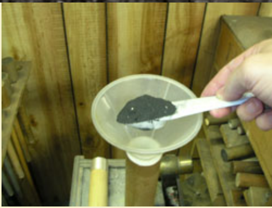
Figure 9: Ramming the driver composition.
