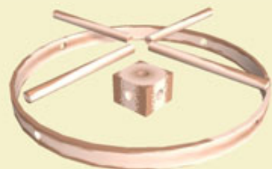
Figure 12: Stitching frame and dowel rods with 2x2 hub.
