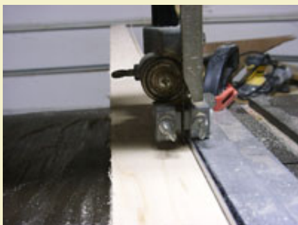
Figure 5: Cutting thin strips of poplar with a bandsaw.
