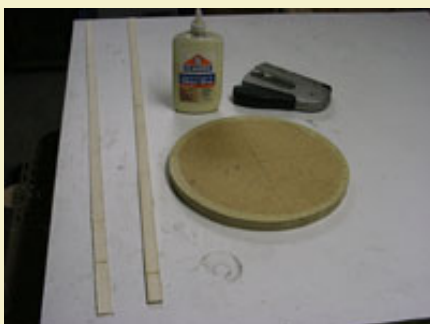
Figure 6: Two thin strips ready to be stapled onto former.
