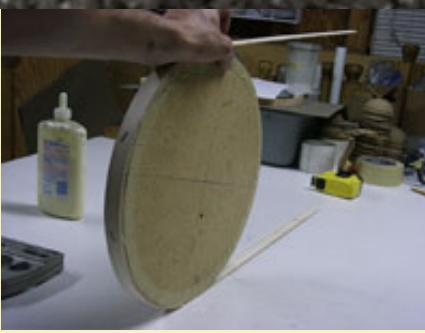
Figure 8: Strips are bent and stapled around former so that the seam for each strip lies directly accross from each other.
