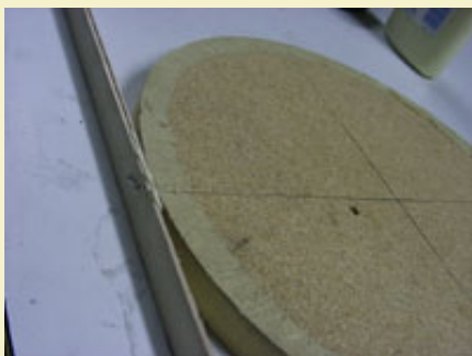
Figure 7: Stapeling halfway overlapped strips to frame at midpoint.
