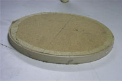
Figure 9: Strips allowed to dry on former, then staples are removed.
