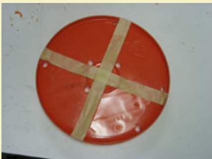
Figure 3: Holes and tape for aid in cutting out quarter panels.
