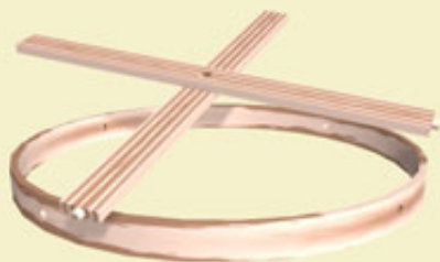
Figure 10: Fitting out the cross members.
