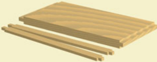
Figure 17: Notching the edge of a solid board before cutting the frame spoke strips from it.
