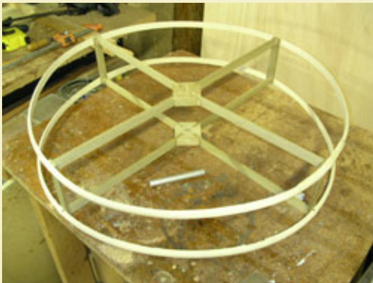
Figure 21: After the top and bottom spokes have been assembled, the axle pin is seated into the hubs.
