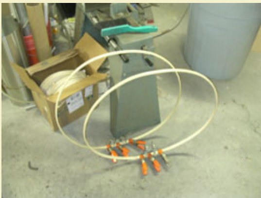
Figure 8: Two clamped hoops waiting for the glue to dry.
