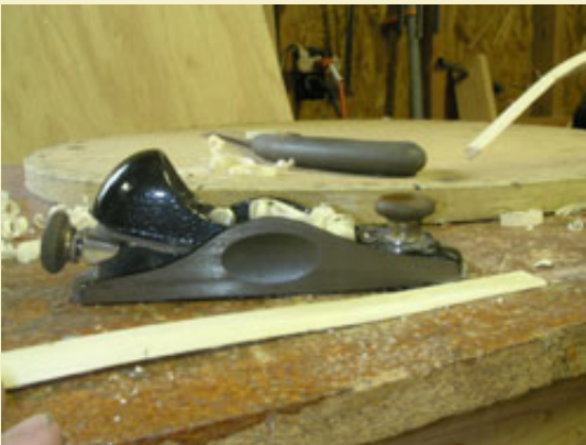
Figure 5: Close-up of gradual 6" long taper.
