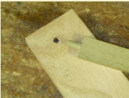
Figure 19: Using a test hole in a scrap of wood to make sure each tenon will fit before installing into the frame.
