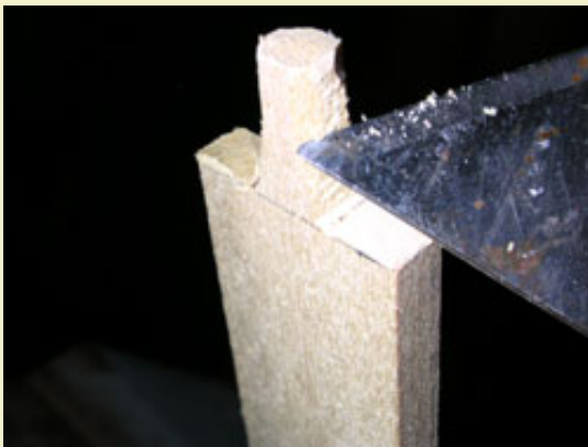
Figure 18: Using a utility knife to round out the square pegs so that they will fit in the mortise holes.
