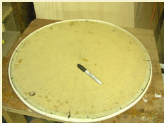
Figure 9: Using the disk template to mark cross member connection points.
