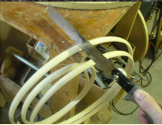
Figure 3: Cutting the reed with a thin pull saw.
