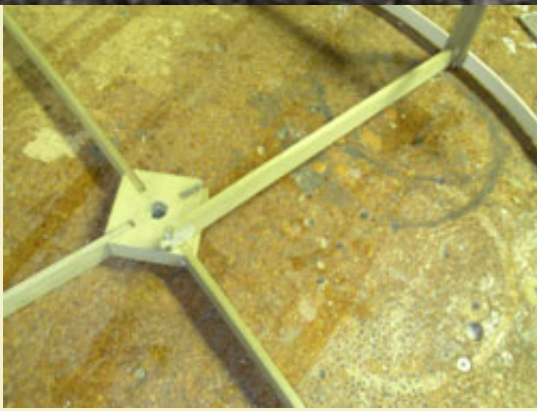
Figure 20: After installing three spokes, the final one is inserted into the hoop and then pulled back and dropped into the slot.
