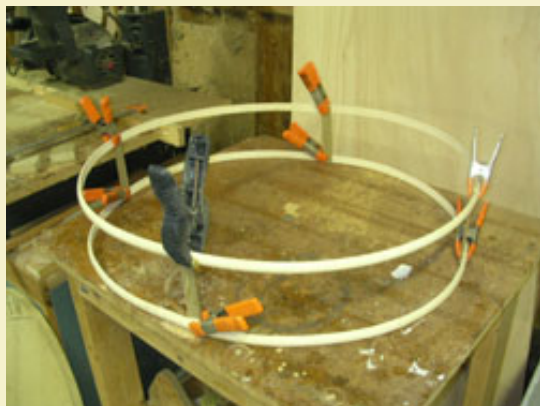
Figure 11: Using spring clamps to hold both ends of all four connectors until glue dries.
