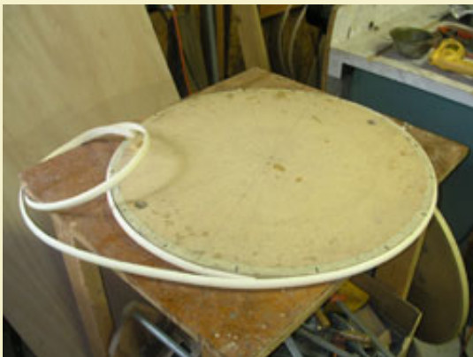
Figure 2: Using a 24" diameter disk to measure out a length of reed for making hoops.
