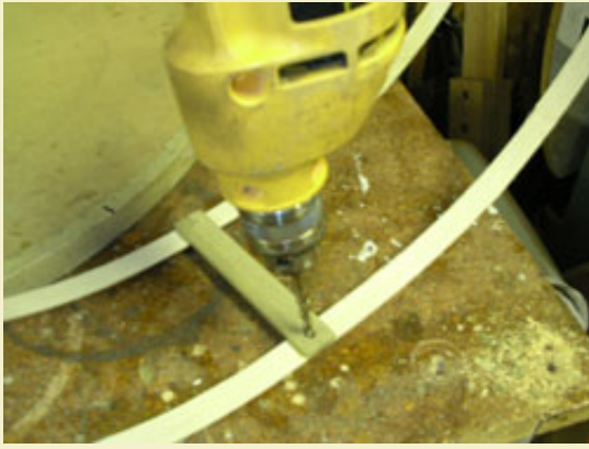
Figure 12: Drilling holes through the vertical cross members where the frame pins will connect into.
