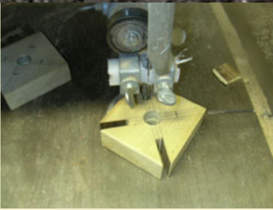
Figure 15: Cutting out the frame junction slots using a band saw.
