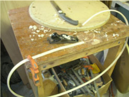
Figure 4: Clamping and planing the rounded side where the ends will be spliced together.
