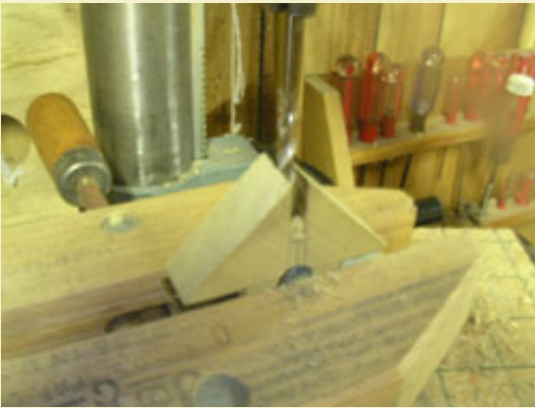
Figure 16: Drilling mortise holes for the frame pins to connect into.
