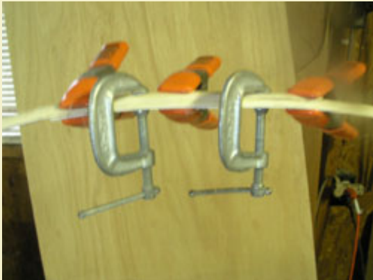
Figure 7: Clamping the ends together to form the overlapping scarf joint.
