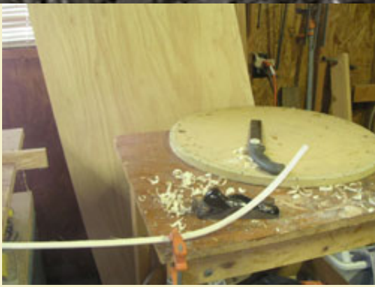
Figure 6: Block planing the flat side of the opposite end.
