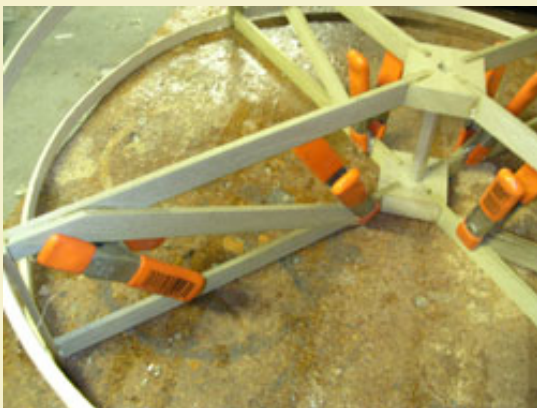
Figure 22: Diagonal braces are glued in place and held with spring clamps until dry.
