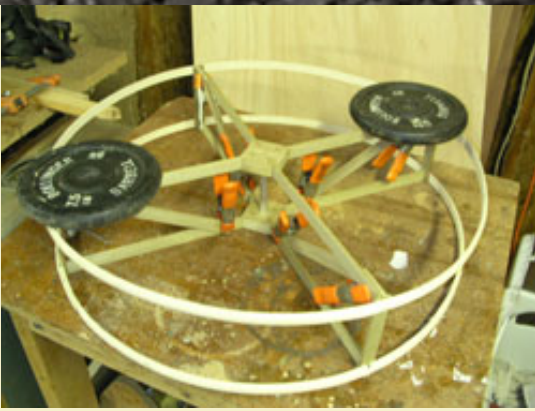
Figure 23: Using weights to make sure the frame lies flat on the table while the diagonal braces are allowed to dry.
