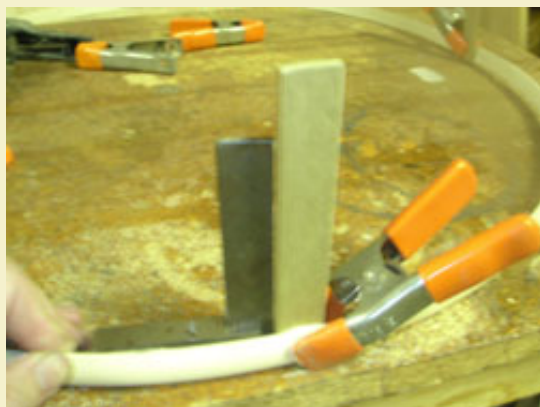
Figure 10: Aligning and gluing the vertical supports that connect the two rings together.
