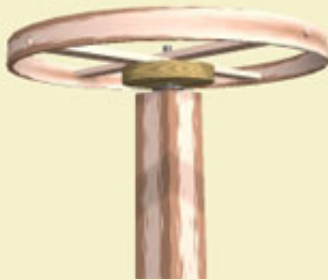
Figure 12: Launch stick with wheel in place.
