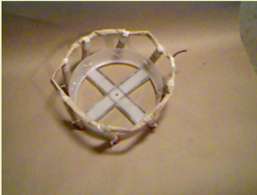
Figure 7: Motors fused together with continuous loop of quickmatch.
