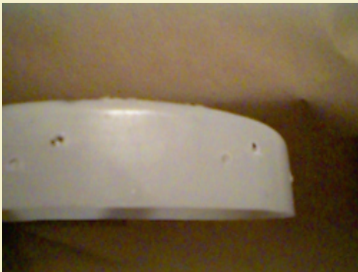
Figure 4: Holes drilled in sides to receive zip ties or wires.
