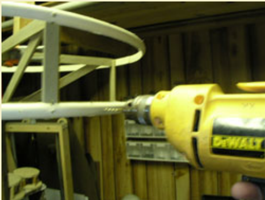
Figure 12: Drilling 3/32" holes through lower ring where tethered lances will be fastened.
