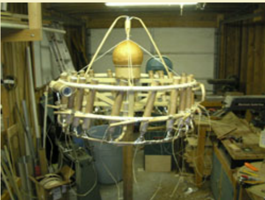
Figure 35: The finished girandola showing the dangling lance strings the way they should look prior to launch.
