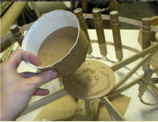
Figure 28: The rim of the shell fixture is slotted and flared out prior to attaching with hot glue.
