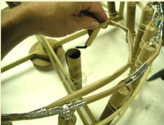
Figure 25: The hooked stick of blackmatch protruding from the quickmatch is inserted into one of the gerbs and tied off.
