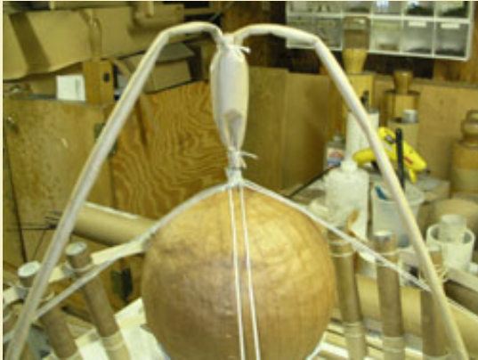
Figure 31: A bucket is tied to the shell's time fuse and matched with dual leaders connected to the main ignition train.
