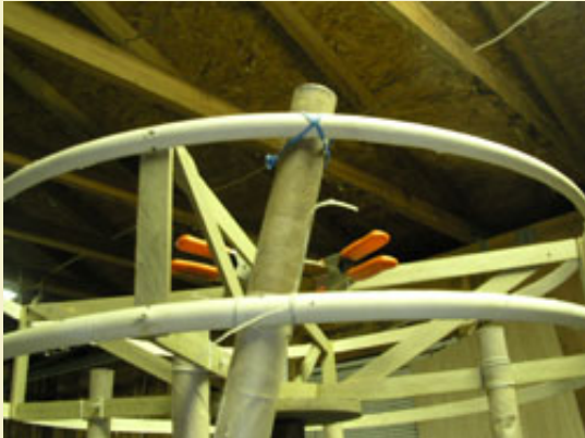
Figure 14: Temporarily holding the top end of a driver using a rubber band while the bottom end is tied.
