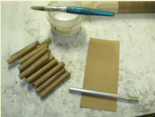
Figure 4: Dry rolling the lance tubes on a 3/8" former.
