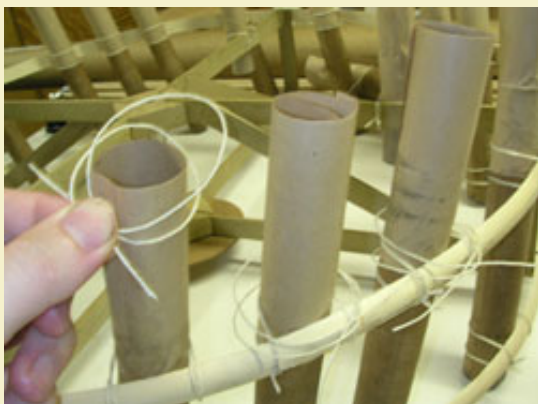
Figure 17: Placing loose clove hitch ties around each driver to be nosed.
