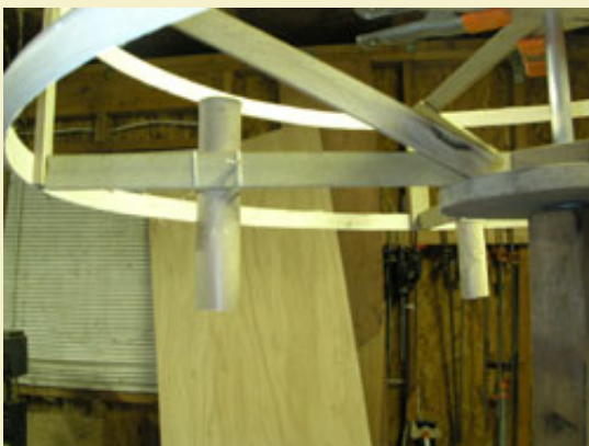
Figure 13: Tying the gerbs onto the lower inside spokes of the frame.
