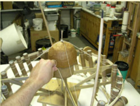
Figure 30: Twine running through the frame members is wrapped around the shell's time fuse for extra reinforcement.
