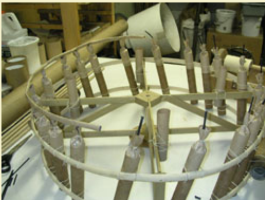
Figure 21: Inserting the driver match into the punched fused pipe.
