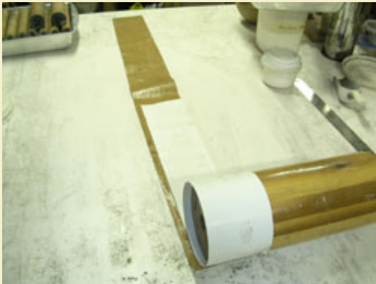
Figure 26: Rolling half of a Maltese style canister to use for a ball shell holding fixture.
