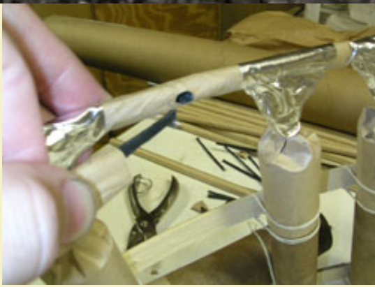
Figure 24: Inserting connections for fusing one of four gerbs.
