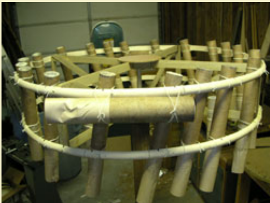
Figure 15: Tying on horizontal drivers after all vertical drivers are attached.
