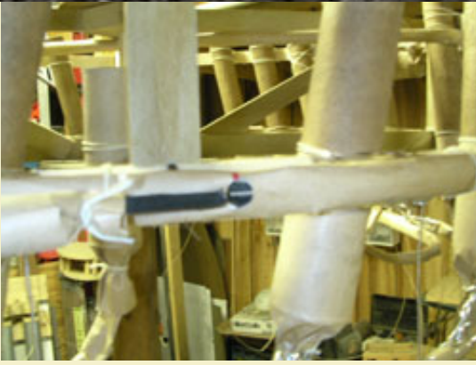
Figure 33: Inserting one of the 16 lances into the ignition ring. Note the dual strands of black match inside the pipe.
