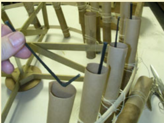
Figure 18: Inserting sticks of black match with a hooked end into each vertical driver.
