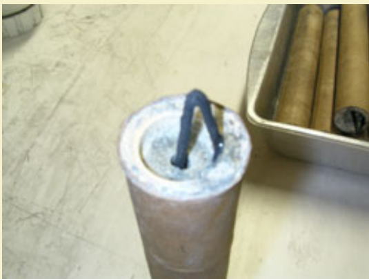
Figure 2: Matching the drivers with a hooked stick of black match secured by a dab of hot glue.
