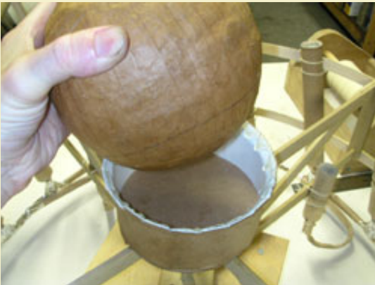
Figure 29: Hot glue is used to secure the 6" ball shell into the holding fixture.
