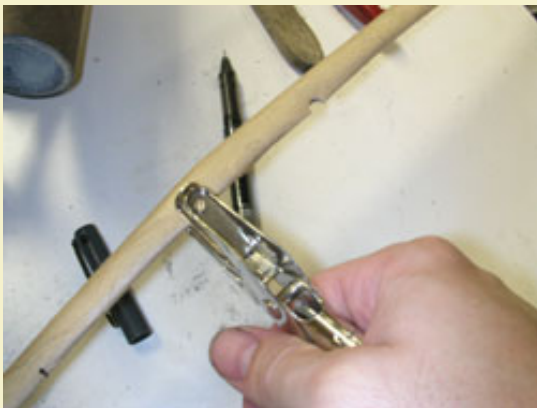
Figure 20: Using a paper hole puncher to open the pipe at the marked connection points.
