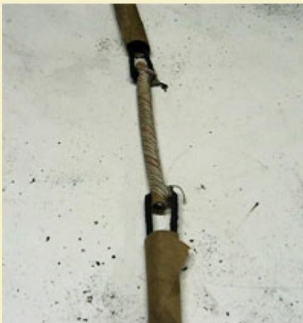
Figure 10: Adding time fuse delay into quickmatch link.
