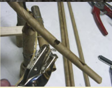
Figure 8: Using a paper punch to make holes in match pipe.
