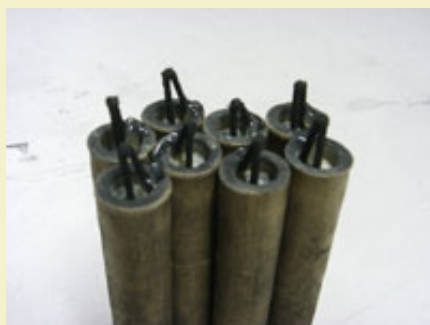
Figure 2: Drivers fuses held in place with hot glue.
