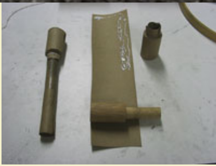
Figure 4: Using a former to make star bag headers.
