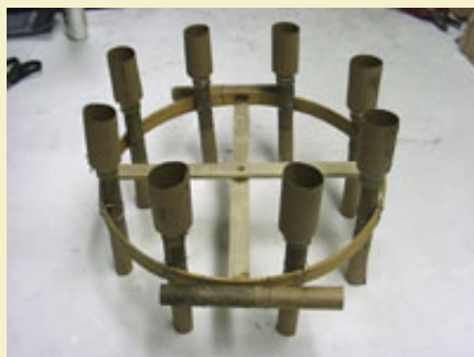
Figure 6: All drivers wired in place prior to fusing.
