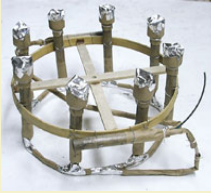
Figure 13: Completed girandola with foil protection covering star bags.
