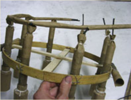
Figure 9: Inserting match sticks into ignition ring.
