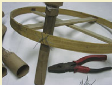
Figure 5: Wiring drivers to frame.
