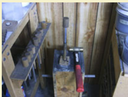
Figure 1: Loading the drivers on a pounding block.
