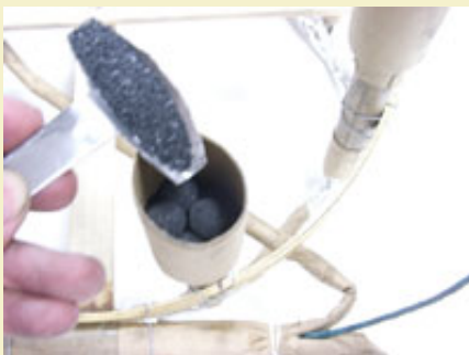
Figure 12: Adding small scoop of 4FA to star bags containing 3/8"
