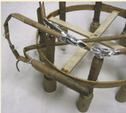
Figure 11: Driver nosing ties in visco, delay link and passfire to other driver.
