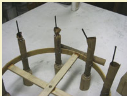
Figure 7: Sticks of black match tied into driver nosings.
