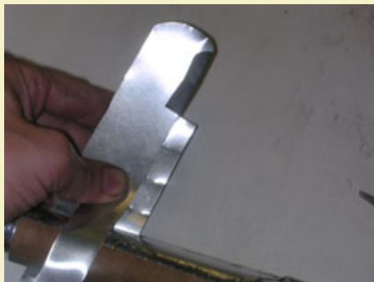
Figure 7: Folding tabs down over the leading edge of the wing.
