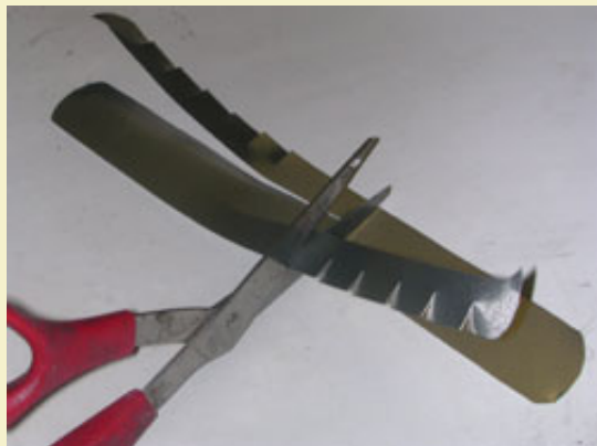
Figure 6: Slotting the tabbed support wings.
