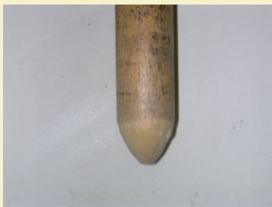
Figure 2: The tapered rammer, key to preventing exhaust hole erosion.
