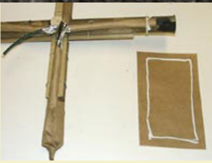
Figure 6: Applying Nosing Paper
