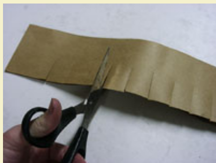
Figure 3: Cutting tabs in the paste strip before pasting.
