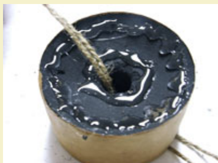
Figure 2: Applying a continuous bead of hot glue around inner and outer edge of comet where it will contact the shell.
