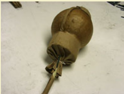
Figure 7: Finishing paper wrapped around comet and leader.
