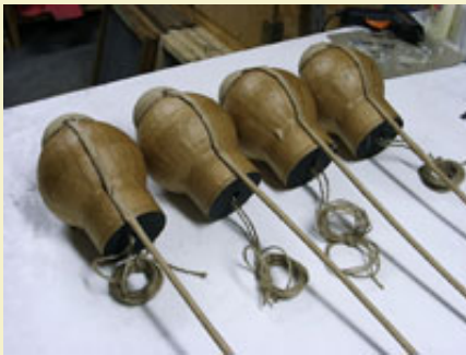
Figure 6: Hot glueing the leaders up the side of the comet.
