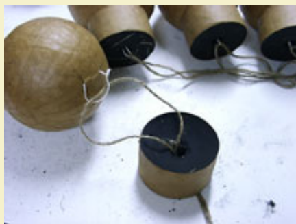
Figure 1: Running the optional lowering cord through the comet.
