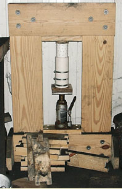
Figure 7: Pressing the comet in a home made wooden frame.
