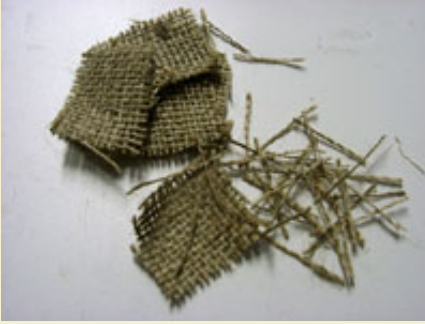
Figure 3: Squares of burlap used to provide the fiber reinforcement.
