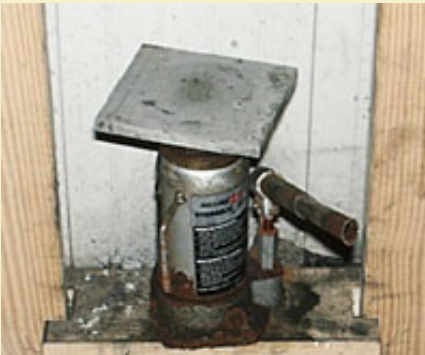
Figure 6: Metal plate on top of 12 ton bottle jack.
