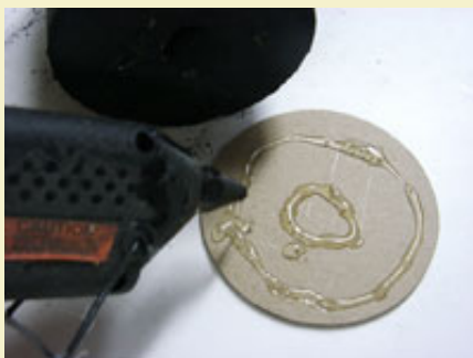
Figure 9: Hot gluing a disk to one end.
