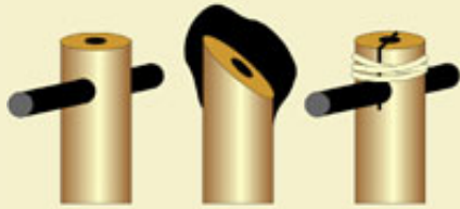
Figure 2: Methods of priming time fuse for taking fire.
