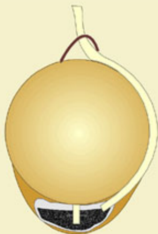
Figure 1: Placing the lift charge in a plastic bag to reduce the potential for water damage.
