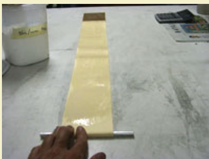
Figure 8: Strips are laid end to end and painted with a 50/50 mixture of white glue and water.
