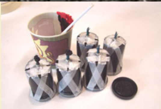
Figure 7: Priming the fuse ends.
