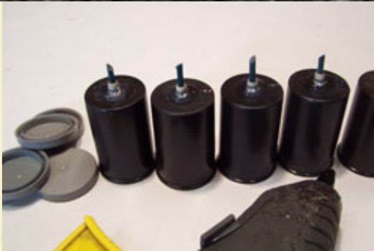
Figure 3: Hot gluing the time fuses in place.
