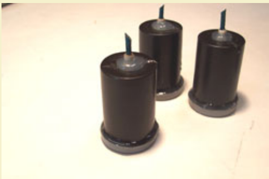
Figure 5: Securing the lids with hot glue.
