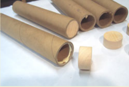
Figure 11: Securing wood plugs into cardboard mortars with wood glue.
