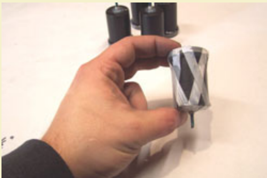
Figure 6: Wrapping with fiber tape.
