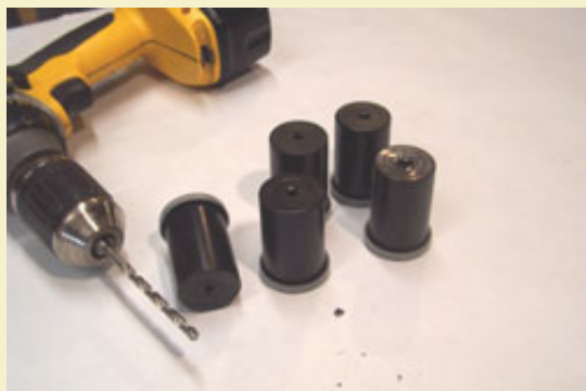
Figure 1: Drilling the fuse holes.
