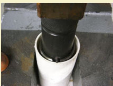
Figure 6: PVC sleeve used as depth stop.
