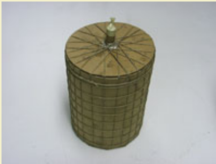
Figure 19: Can is spiked with flax twine as for an Italian shell.
