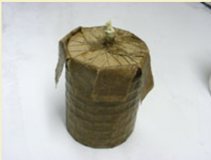
Figure 20: Pasting an initial 30lb wrap to insure a good gas seal.
