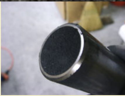
Figure 7: Composition shaved flush with end of pump after pressing.
