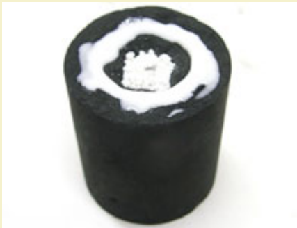
Figure 12: Cavity filled with whistle mix and glued around rim.
