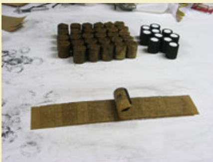
Figure 13: Pasting in crossettes from a stack of pasted strips.
