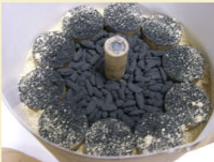
Figure 17: BP on puffed rice break charge filled in around a spolette.
