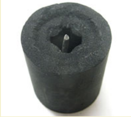
Figure 11: Chinese fuse inserted and cut flush with top of cavity.
