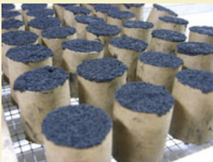
Figure 14: Primed ends dipped in 4Fg insures ignition.
