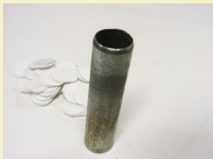
Figure 8: Tapered 1" conduit used as disk punch.
