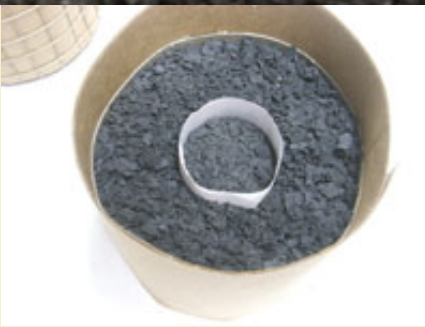
Figure 10: 2FA is loaded into burst core, while rough powder is used to fill the remaining space above the insert shells.
