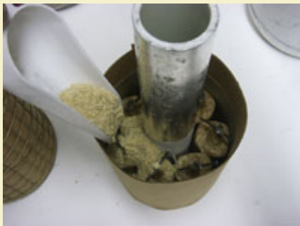
Figure 8: Packing sawdust into the gaps between the shell wall and canulle.
