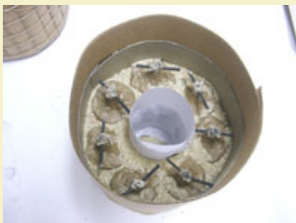
Figure 9: Sawdust fully loaded and canulle is removed.
