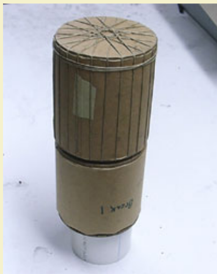
Figure 12: The second break is inserted upside down into the hole in the bottom of the first break.
