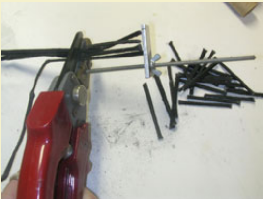
Figure 4: Using the anvil cutter with length gauge set to 2" for cutting 70 sticks of black match.
