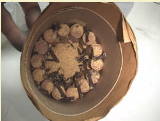
Figure 10: Loading rows of 14 pill box stars, using sawdust to pack in the gaps behind them.
