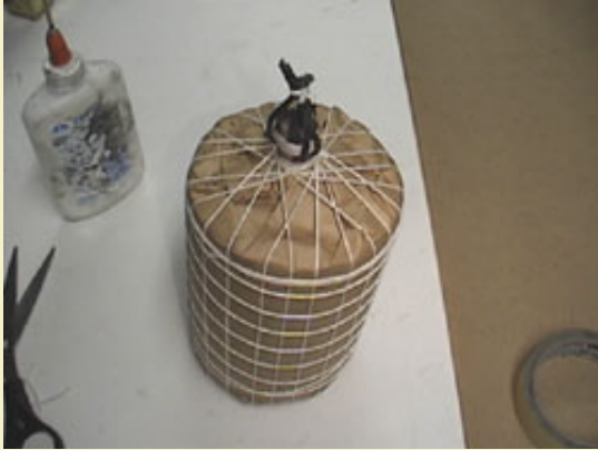
Figure 13: This shell was finished using unpasted paper followed by another layer of spiking, known as the "rinfasciature" method.
