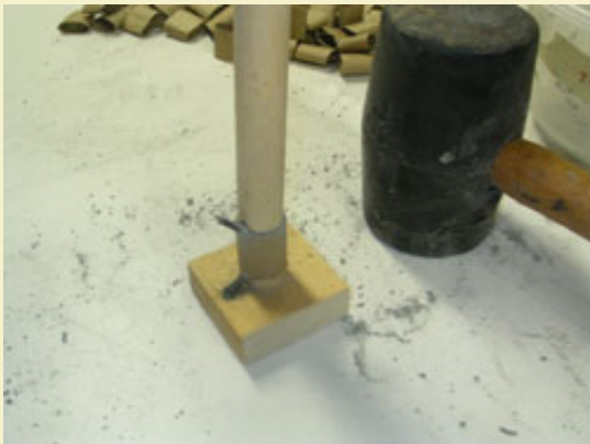
Figure 8: A couple of light taps from a rubber mallet for additional consolidation.
