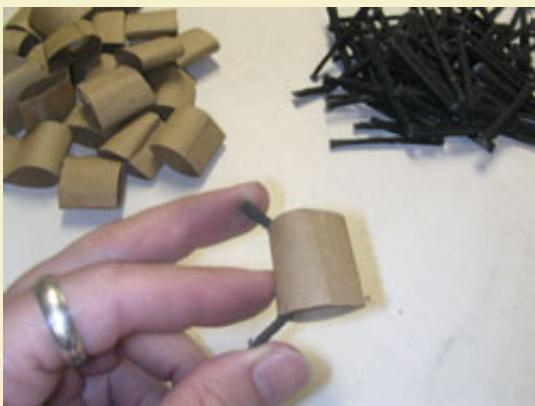
Figure 5: Inserting a stick of match and bending the ends to hold it in place during loading.
