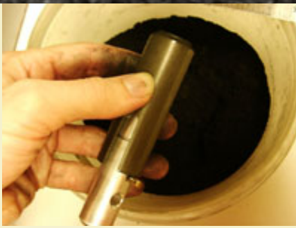
Figure 6: Push pin down to sleeve and cut off excess comet.
