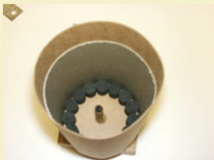
Figure 8: Loading in the first row of comets.
