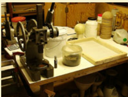
Figure 3: Arbor press, comet pump, comp bucket and drying screen.
