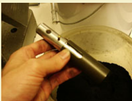
Figure 4: Keep pin 1/2" - 3/4" above sleeve when loading.
