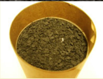
Figure 11: Remaining space filled with rough powder.
