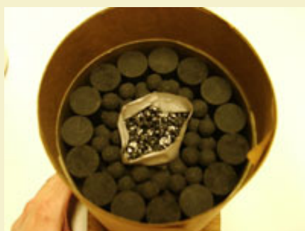
Figure 10: Center filled with break charge and round color stars.
