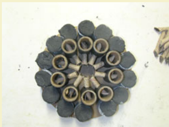
Figure 5: Determining maximum possible time fuse length.
