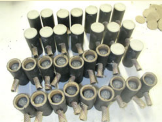
Figure 10: Padding the remaining space with powdered clay prior to gluing on second end disk.
