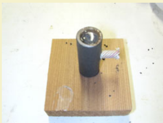
Figure 13: Hot glue used to fill ends of tube.
