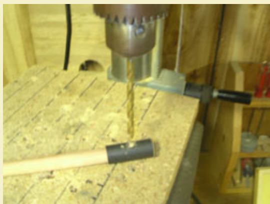
Figure 4: Drilling 7/32" time fuse holes at center of scatter star casing.
