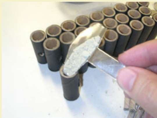
Figure 8: Padding with powdered clay. Note home-made scoop for easy loading without funnel.
