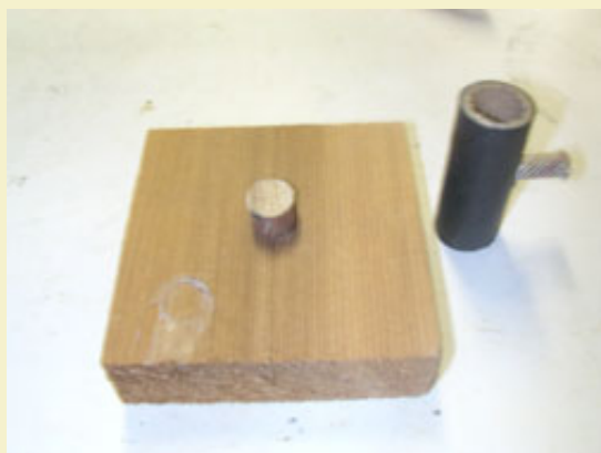
Figure 12: Loading fixture for the hot glue method.
