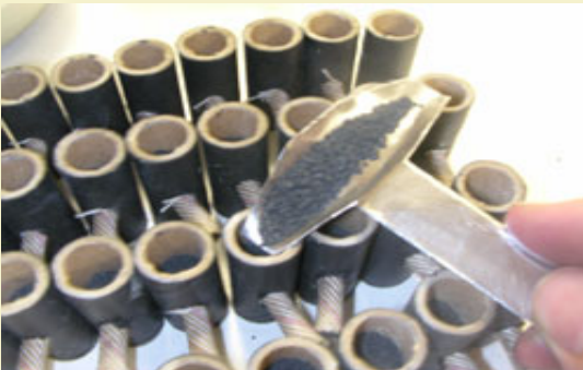
Figure 9: Adding center charge of 2Fg after inserting 1st star and time fuse.
