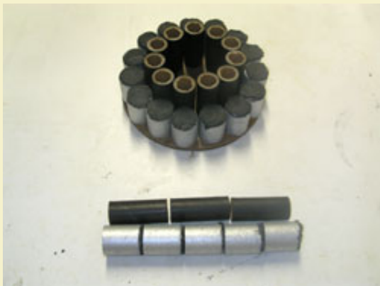
Figure 3: Trial fitting shell components onto a 4-1/2" dia. disk.
