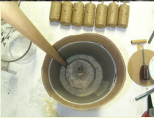
Figure 34: Tamping sawdust tightly around the bottom shot.
