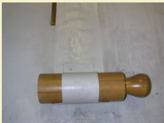
Figure 3: Centering the inner case when rolling the outer case.
