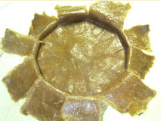
Figure 45: Folding the tabs down in two separate layers.
