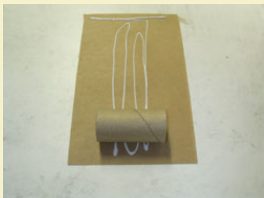
Figure 21: Rolling the outer wrap.
