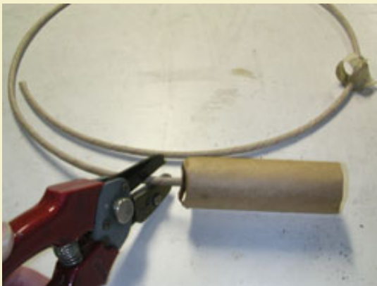
Figure 25: Cutting time fuse to proper size.
