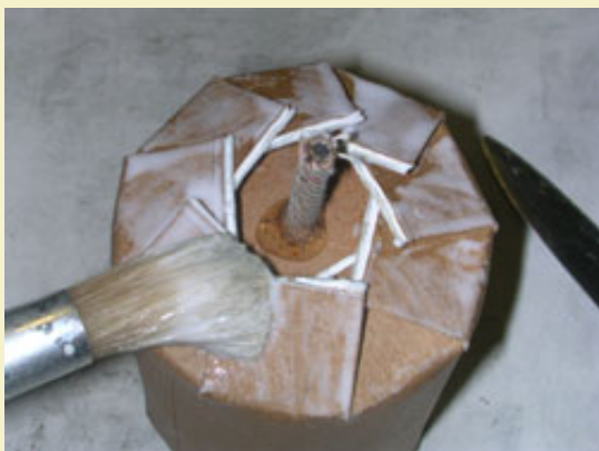
Figure 16: Painting white glue over top tabs.
