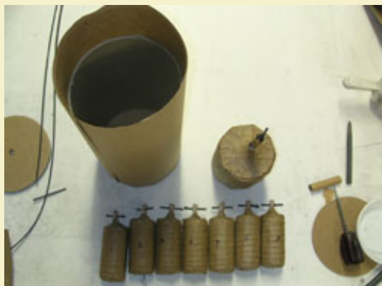
Figure 32: Shell case with components ready to load. Note the sequence numbers have been written on the reports.
