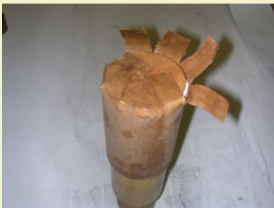
Figure 8: Pleating down the second set of tabs.
