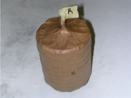
Figure 19: Pasted bottom shot is dried and ready for cross matching.
