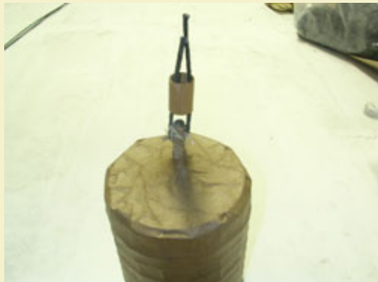
Figure 33: Retainer sleeve on the long cross-match of the bottom shot.
