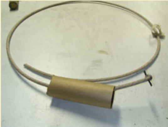
Figure 24: Thread case onto time fuse coil before cross-matching.
