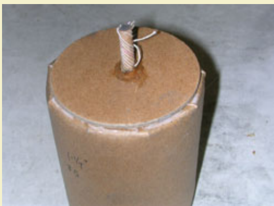
Figure 17: Hot glue sealed around time fuse base.
