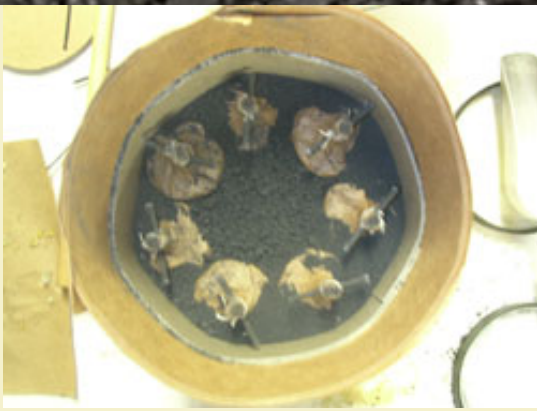
Figure 37: Filling all open spaces with fast burning 1/8" rough powder.
