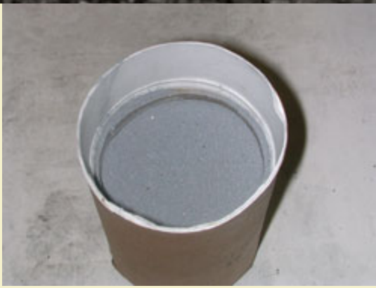
Figure 11: Filled with 70/30 flash.
