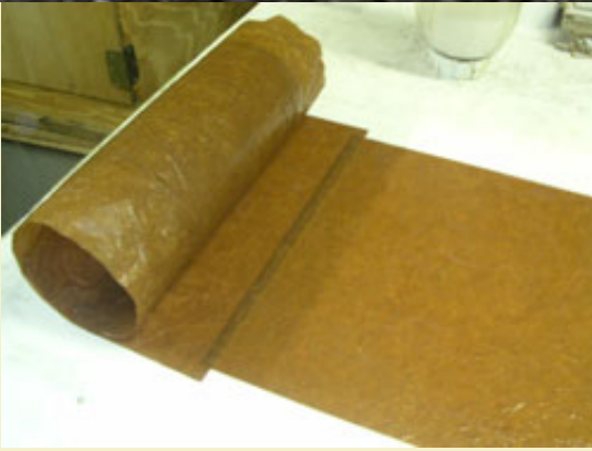
Figure 43: Pasting in with 4 or 5 turns of 70 lb virgin kraft.
