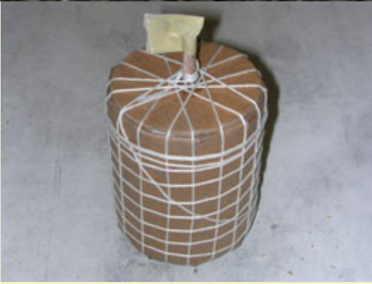
Figure 18: Spiked with 8 ply linen twine.
