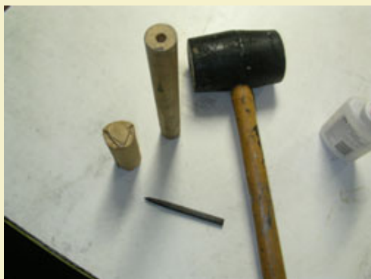
Figure 22: Tools for punching the fuse hole.
