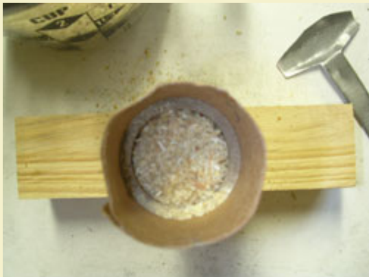
Figure 27: Sawdust pressed above flash charge.
