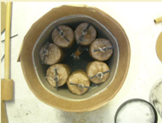
Figure 36: Reports loaded tightly in a ring.
