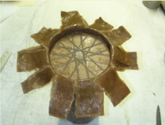
Figure 44: Tearing the tabs by hand.
