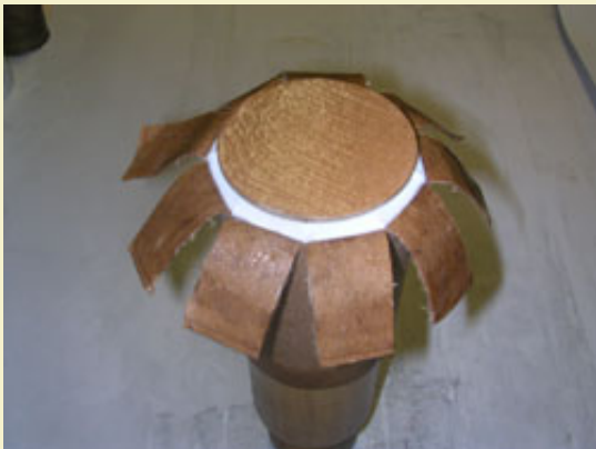
Figure 6: Pleating the first set of tabs.
