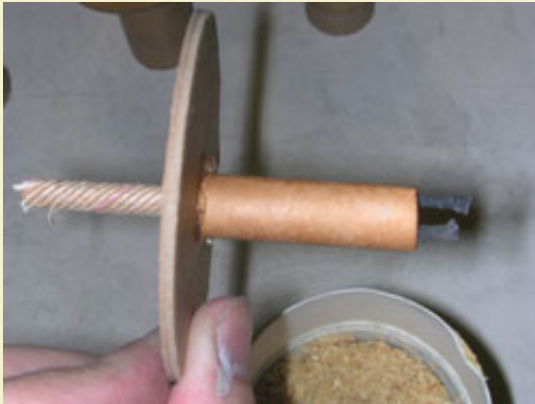
Figure 13: Fused disk ready to close the can.
