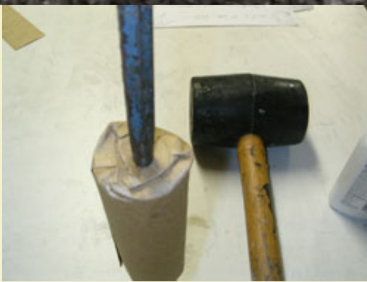
Figure 23: Punching the fuse hole.
