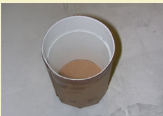
Figure 9: Dried bottom shot can ready to load.
