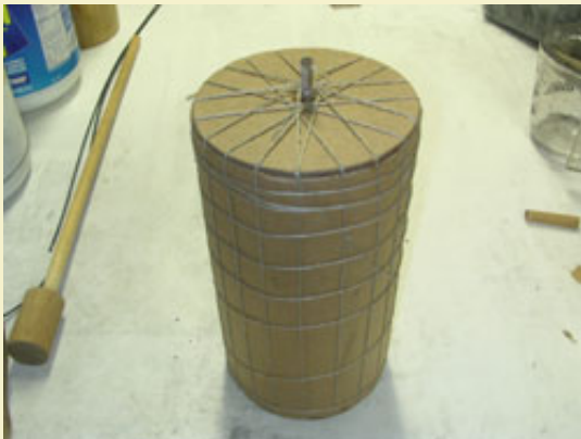
Figure 42: Spiked with high quality flax twine.
