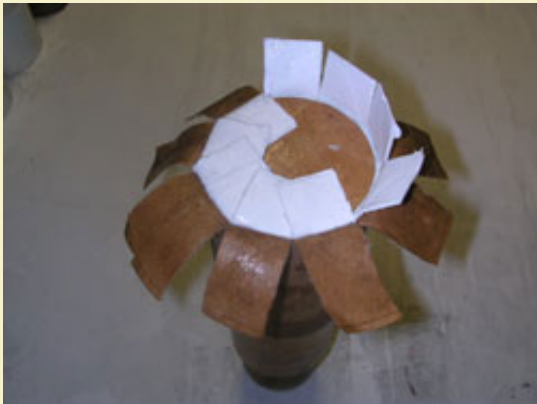
Figure 6: Pleating the first set of tabs.
