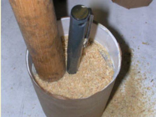
Figure 12: Tamping sawdust above the flash.
