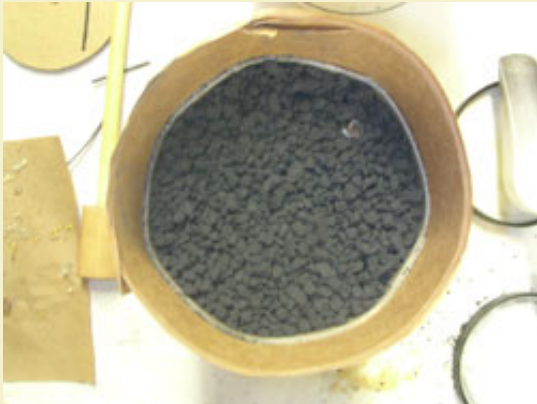
Figure 38: Leveling the space above the reports with 1/4" rough powder.
