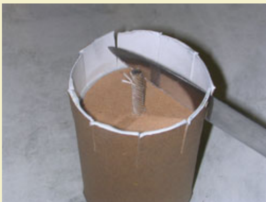
Figure 15: Slicing the tabs on the top side.
