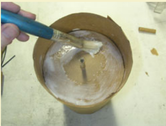
Figure 39: Using white glue when pleating over the end disk.
