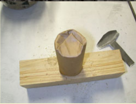
Figure 30: Completed third fold of triangle fold.
