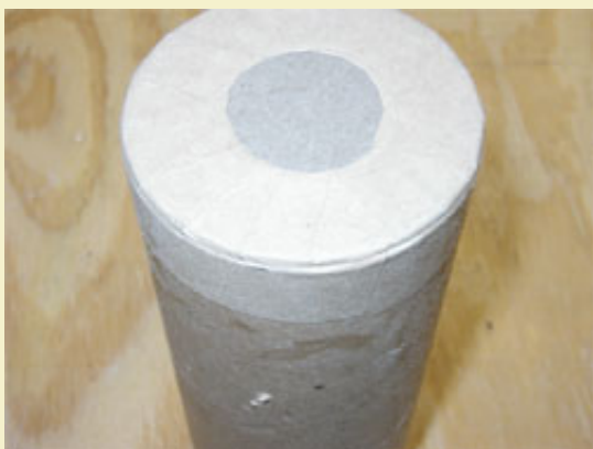
Figure 3: Pleated paper over bottom of the can.
