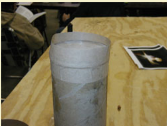
Figure 4: Piston made with wadding between two solid disks.
