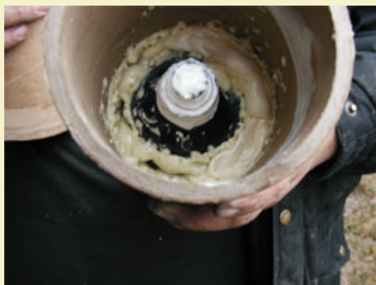
Figure 2: Foam seal around the 1 Liter bottle.
