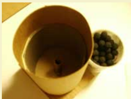
Figure 5: Chipboard liner in place.
