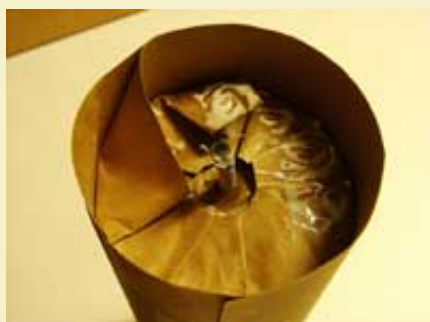
Figure 4: Pleating over the end disk.
