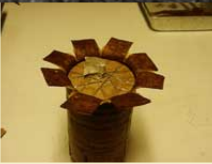
Figure 12: Pasting in over the end disks.
