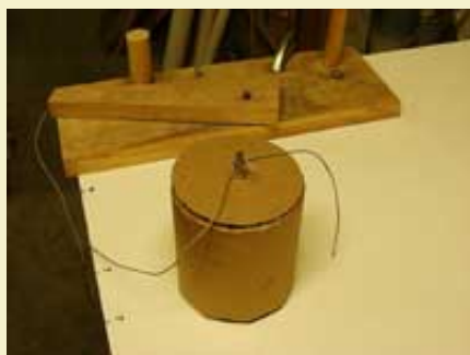
Figure 9: Flax twine tied off to time fuse.
