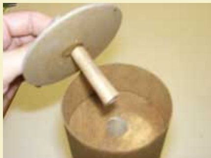
Figure 3: Inserting the fused end disk.
