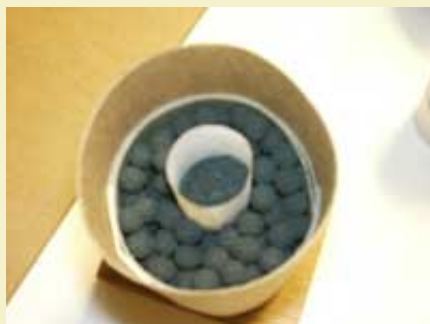
Figure 7: Stars and burst charge loaded.
