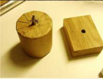
Figure 8: Shell ready for spiking.
