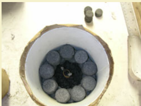
Figure 13: Loading two rows of comets on top of the rough powder.
