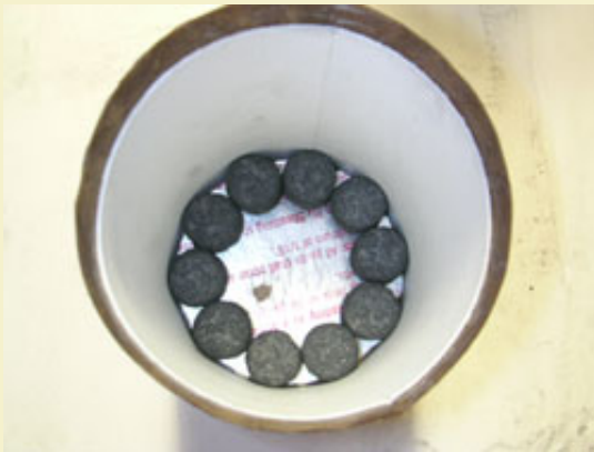
Figure 15: Loading comets into the single color break shells.
