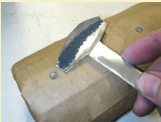
Figure 39: Charging the pipette with 2Fg black powder.
