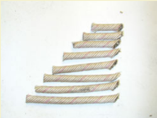
Figure 38: Increasing series of time fuses cut for each break.
