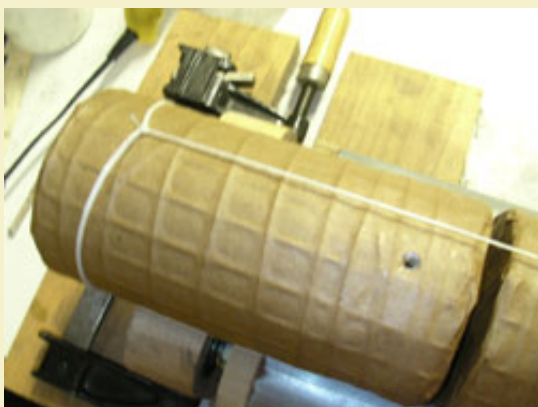
Figure 29: Starting the spiking twine at one end.
