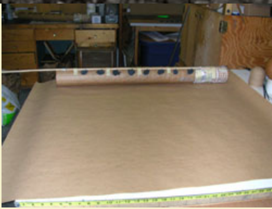
Figure 46: Rolling the outer wrap around the shell.
