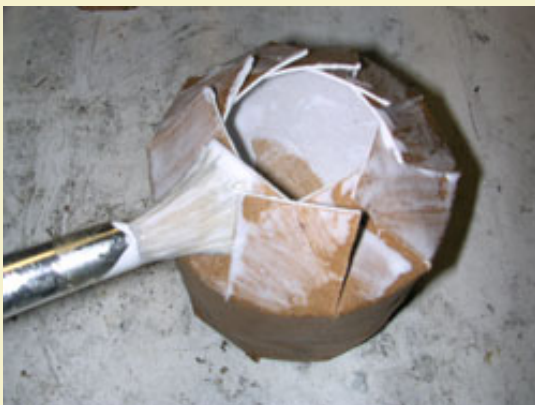
Figure 20: Tabs are glued and folded down over the end disk.
