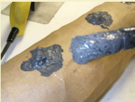
Figure 42: Priming the time fuse.
