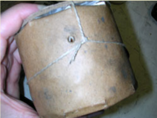
Figure 22: Starting the spiking twine with knot located next to fuse hole.
