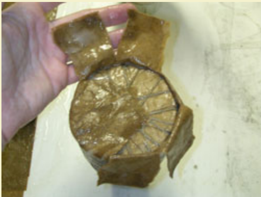
Figure 26: Ends are pasted by folding over tabs torn in the overhanging paper.
