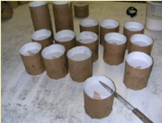
Figure 19: Slicing the tabs for closing the shells.
