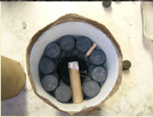
Figure 14: The third row of comets contains the pipette glued to the shell wall.
