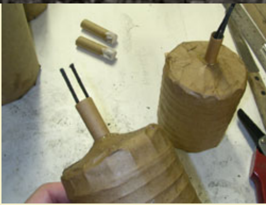
Figure 9: Holding the match with a retaining tube to keep it centered.
