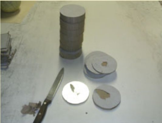
Figure 4: Separating the disks after cutting.
