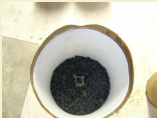
Figure 12: Placing a layer of rough powder on top of the bottom shot.
