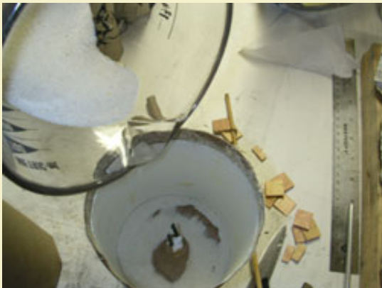
Figure 11: Dusting in the bottom shot with sand.
