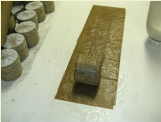
Figure 25: Pasting two layers of 30lb recycled kraft onto each break.
