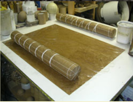
Figure 36: Finished shell being pasted in.
