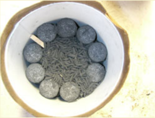
Figure 18: Close-up of shell loaded with 7:1 KP on rice hull break charge.
