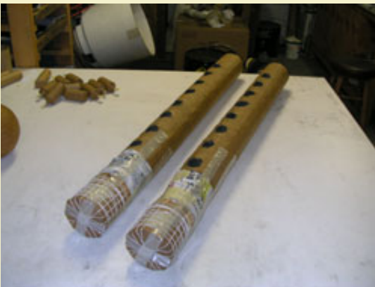
Figure 45: Lift components held in place with fiber tape.
