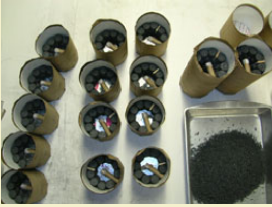
Figure 17: All the breaks are loaded, dried and ready for break charge.
