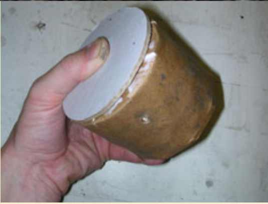
Figure 21: A second end disk is placed over the tabs.
