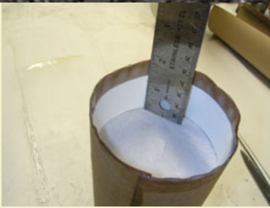
Figure 6: Leaving 1.5" of poster board above the end disk.
