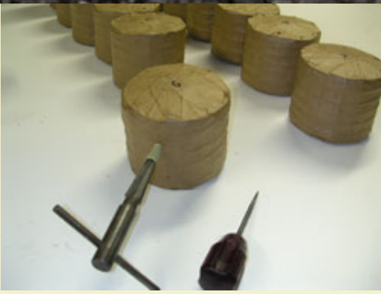
Figure 27: Re-punching the fuse holes after the pasted paper dries.
