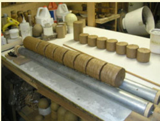
Figure 28: Aligning the shells on a Maltese Shell Roller.
