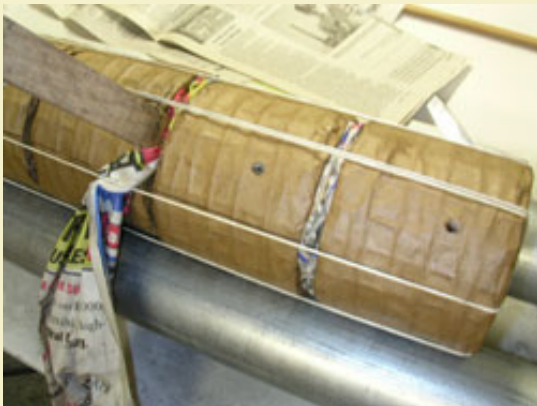
Figure 32: Ramming damply pasted newspaper between the breaks.
