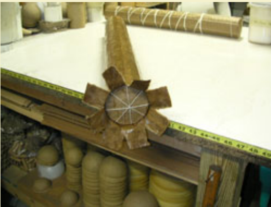
Figure 37: Pasting over the ends of the shell.
