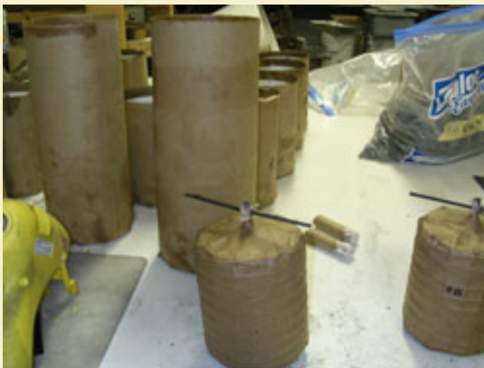
Figure 8: Cross matching the bottom shots with extra long match.
