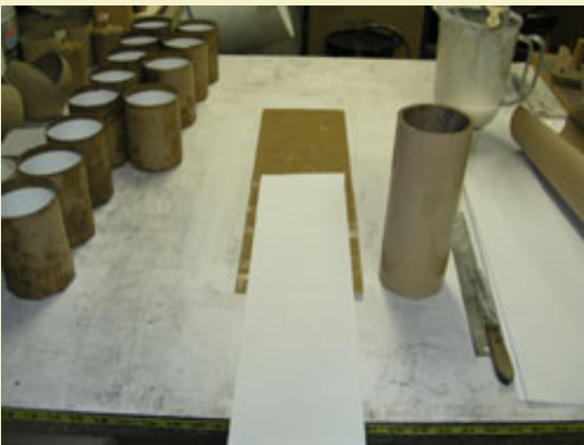
Figure 5: Rolling the shell cans.
