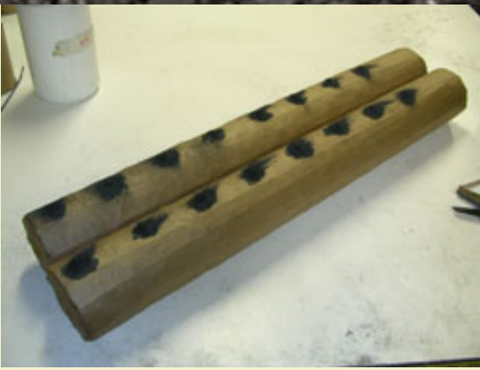
Figure 43: Primed and dusted fuse tips on two shells.
