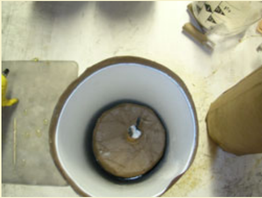
Figure 10: The bottom shot loaded into the last break.
