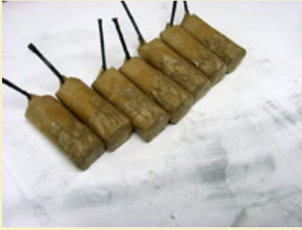
Figure 5: Pasted paper over bottom protects against gas leaks.
