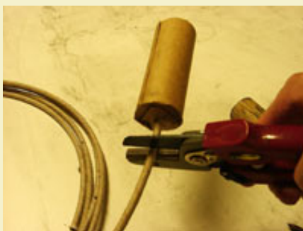
Figure 9: Time fuse is pulled through and cut where marked.
