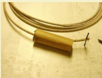
Figure 8: Case threaded onto time fuse coil and crossmatched.
