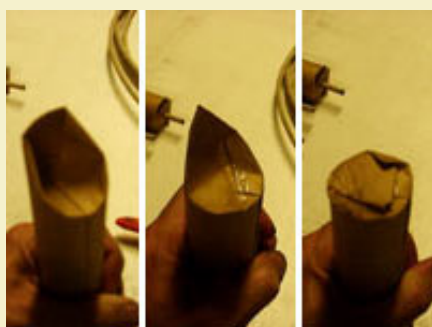
Figure 5: Making the triangle fold.
