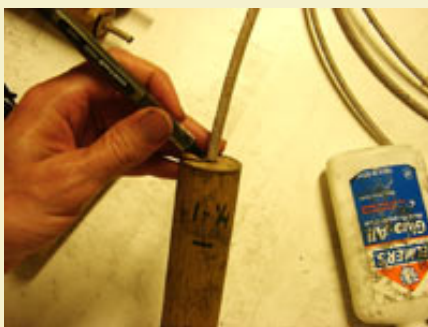
Figure 7: Using a length gauge to mark time fuse.
