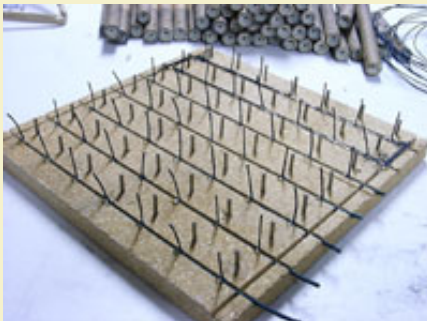
Figure 6: Launch board is fused up and ready for Z-bomb installation.
