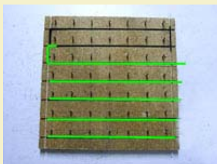
Figure 3: Main body visco path (green) and black match finale path (black).
