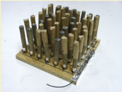
Figure 11: Foil tape used to seal and protect the black match ignition strip.
