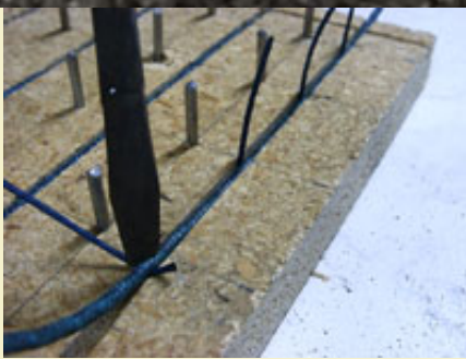
Figure 4: Locking in the 1/16" mini visco with 1/8" visco.
