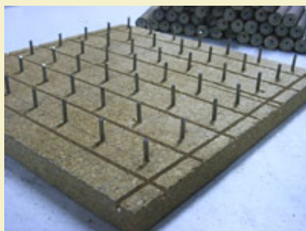
Figure 2: 1-1/2" roofing nails with points cut off.
