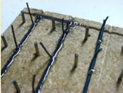
Figure 5: Hot glue applied over black match paths to protect from accidental ignition.
