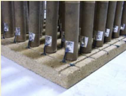
Figure 8: Securing fuse with a patch of foil tape.
