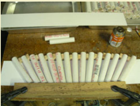
Figure 6: All 15 tubes glued into place on one of four plates.
