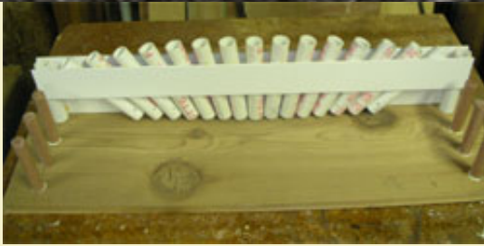
Figure 13: Shot rows slide onto support pins.
