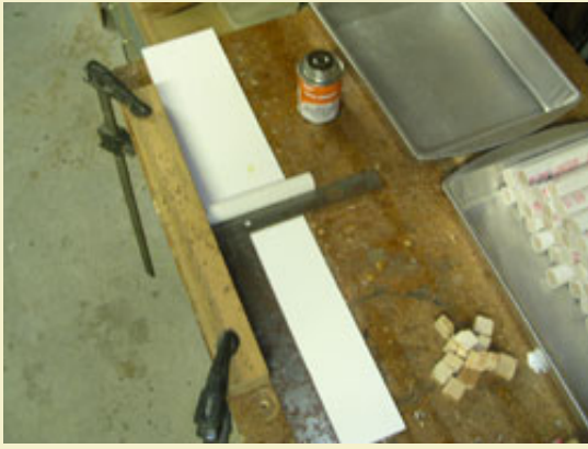
Figure 4: Using a wood alignment fence and an framing angle to mark the center tube.
