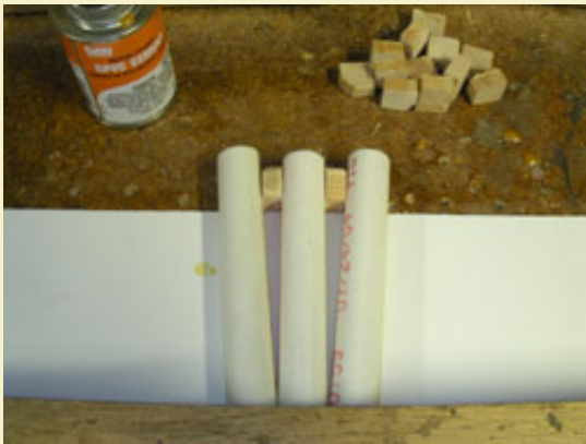
Figure 5: Using small 1/2" spacer blocks to set tube angles.
