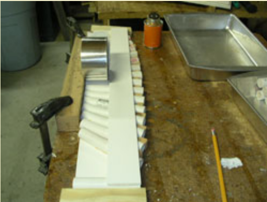
Figure 8: Gluing the front PVC strip across all tubes to finish the plate.
