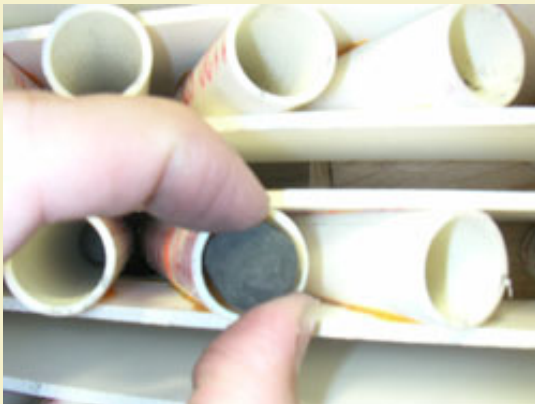
Figure 22: Inserting a 5/8" round star.
