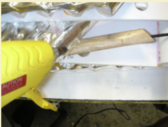
Figure 19: Using hot glue to connect piped match segments.
