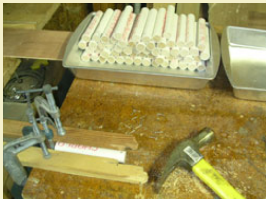
Figure 3: Bracing the tube while tacking the wood plugs in place.
