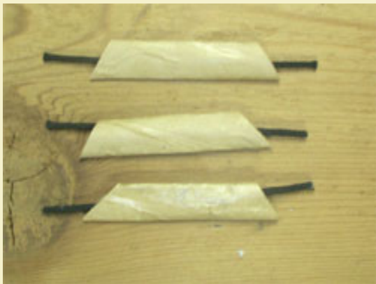
Figure 18: Piped match segments for connecting the rows together.
