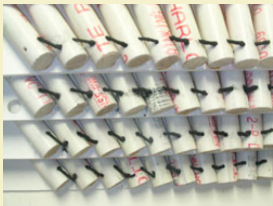
Figure 15: Fusing shots together with segments thin blackmatch.
