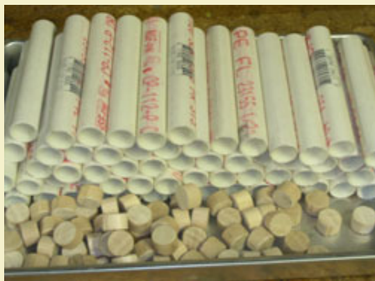
Figure 1: 60 tubes and end plugs ready for assembly.
