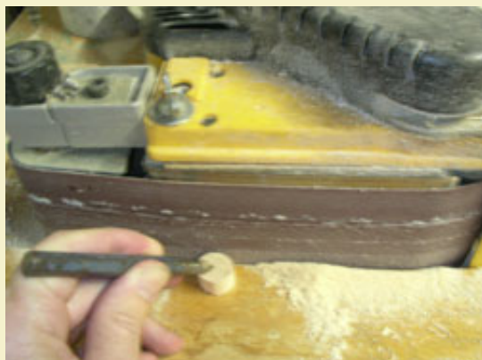
Figure 2: Using a belt sander to trim down wood plugs that are too large.
