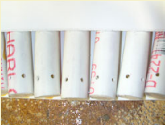
Figure 10: Drilled out 1/8" passfire holes.
