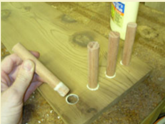
Figure 12: Gluing wood pins onto the holding fixture.
