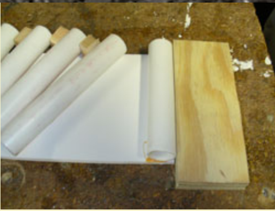
Figure 7: Attaching the guide tubes at each end.
