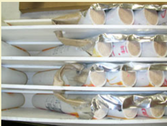
Figure 20: Piped match connecting the rows together.
