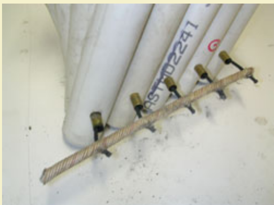
Figure 18: Inserting parallel blackmatch sticks into brass pipes.
