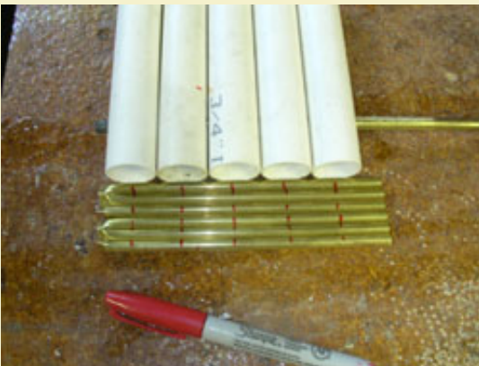
Figure 10: Aligning fuse tubes in front of mortars and marking passfire holes to be drilled.
