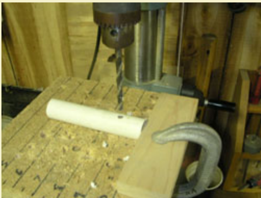
Figure 6: Drilling 1/4" fuse pipe holes 1-1/8" from bottom of pipe. Note use of stop block to eliminate the need to measure each hole location.
