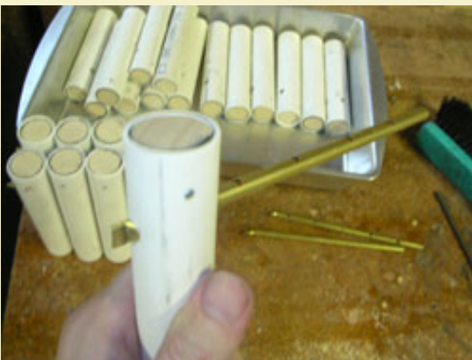
Figure 13: Sliding mortars on to the fuse pipes.
