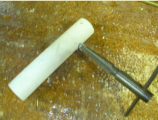
Figure 12: Slightly enlarging fuse pipe holes with a hand reamer prior to assembly.
