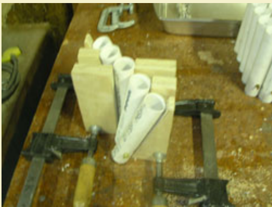
Figure 15: Two angle fixtures are used to align the tubes while hot glue is applied to fix them in place.
