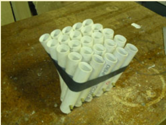
Figure 16: The five rows of angled tubes are finally banded together using PVC cement between the tubes to secure them into one solid block.
