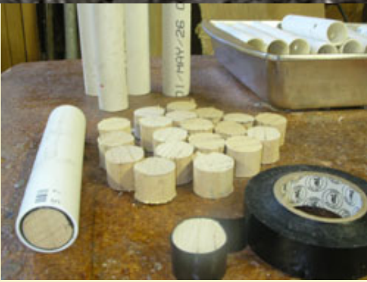
Figure 7: Plugging bottom of tubes with 3/4" long wood plugs cut from a 7/8" dowel rod. A snug fit is obtained by wrapping 4-5 turns of electrical tape around each plug.
