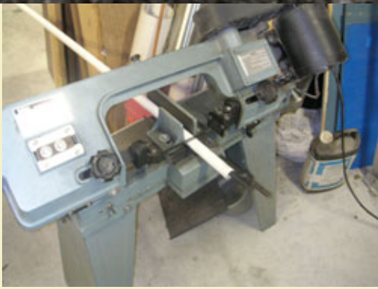
Figure 4: A vertical bandsaw makes cutting PVC mortars fast and easy.
