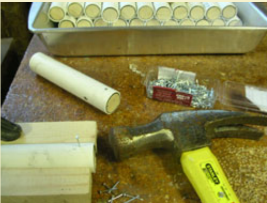
Figure 8: Using two small nails to hold each plug into the tubes.
