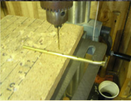
Figure 11: Drilling passfire holes with a 3/32" bit.
