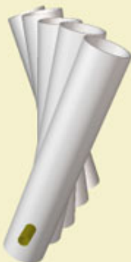
Figure 2: A more efficient fan configuration aligned on a common axis.
