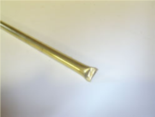
Figure 9: One end of each 6" long brass tube is pinched closed using a vise or pliers.
