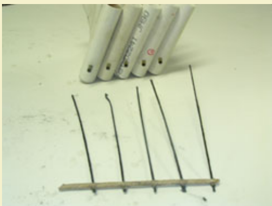
Figure 17: Crossmatching one continuous piece of time fuse.
