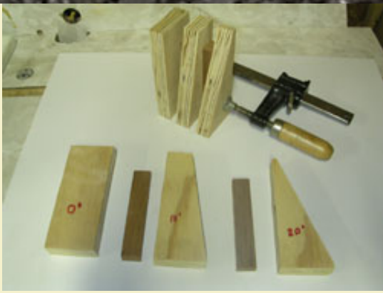
Figure 14: Building the angle fixture used to hold the mortars at the proper angles during gluing.
