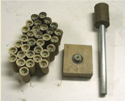
Figure 4: Clay plugs rammed and drilled.
