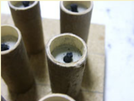
Figure 5: Chinese fuse inserted through passfire hole.
