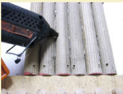
Figure 14: Glueing each row of tubes together before fusing.
