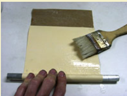
Figure 2: Applying diluted white glue to paper before rolling.
