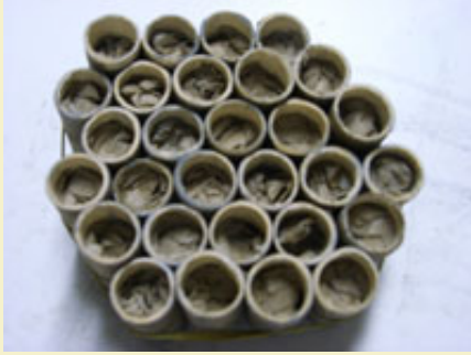
Figure 8: Paper wadding stuffed into tubes.
