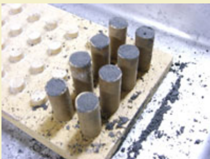
Figure 6: Damp color comp pressed into end cavity.
