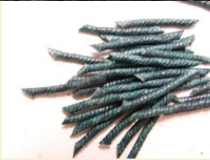
Figure 15: Cutting visco at a sharp angle to increase its ability to take fire.
