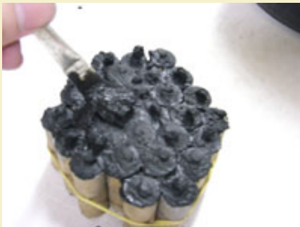
Figure 10: Brushing a prime slurry onto the dried color comp.
