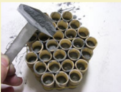
Figure 7: Loading flash into tubes with special scoop.
