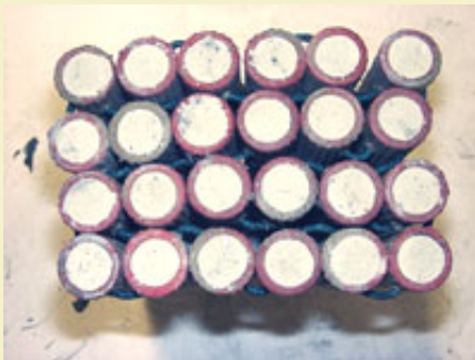
Figure 17: Bottom view after all tubes are fused together.
