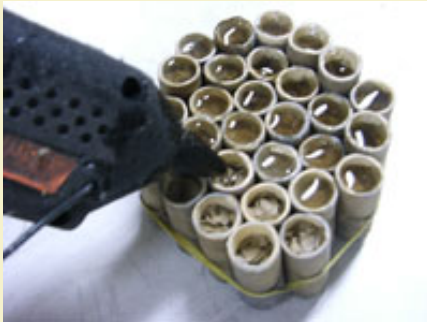
Figure 9: Sealing ends with hot glue.
