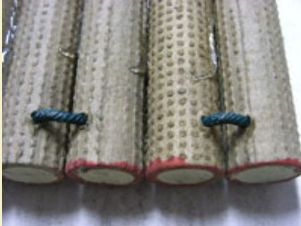
Figure 16: Closeup of visco fuse links.
