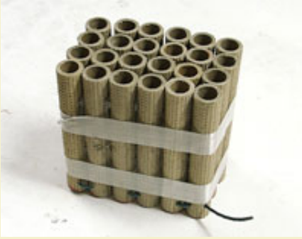
Figure 19: Finished cake held together with a few bands of fiber tape.
