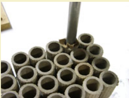
Figure 18: Pushing in retainer wadding after all shots are loaded.
