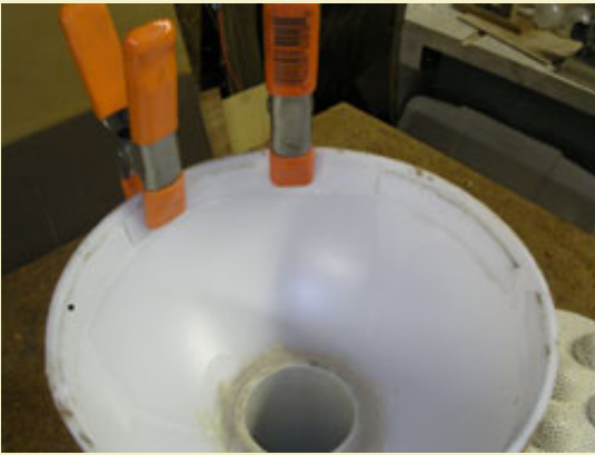
Figure 4: Converting an 8" male hemi into a female hemi.
