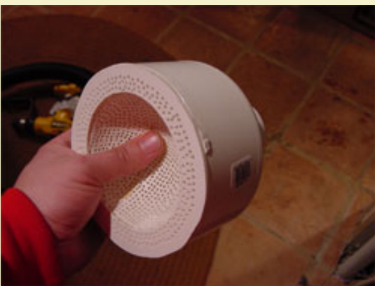
Figure 6: PVC endcap used to house a 4" mold.
