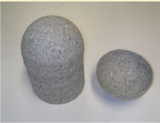
Figure 8: 6" hemis made from the shredded newspaper insulation.
