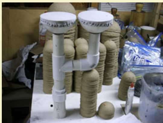
Figure 1: Multi-mold for producing two 4" hemis at once.
