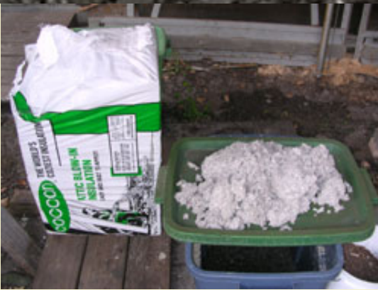
Figure 7: Blown-in insulation eliminates the blender process for making the paper mulch.
