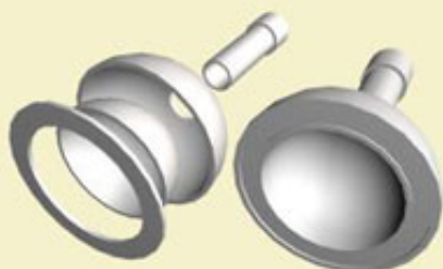
Figure 2: Mold made from plastic shell hemis, PVC and a plastic ring.
