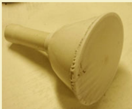
Figure 4: An 8" mold with filter cap in place. Outer casing was made from a flower pot.
