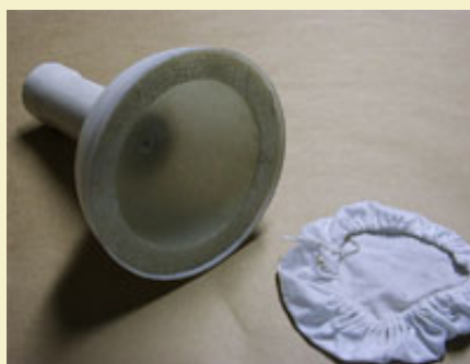
Figure 3: A 6" fiberglass mold with spandex filter cap.
