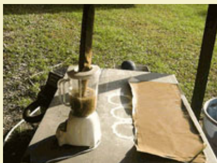
Figure 8: Mulching recycled kraft in a blender.
