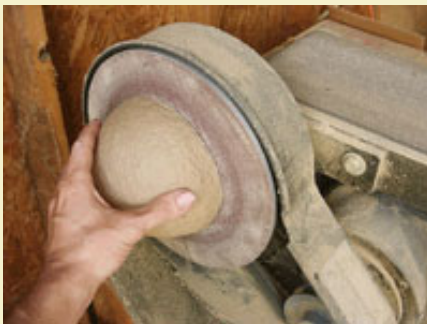
Figure 16: Cleaning up the edges on a disk sander.
