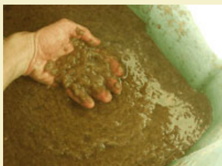
Figure 9: Mulched paper diluted with water.
