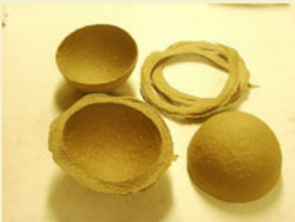
Figure 15: Cutting the flange off of dried hemis.
