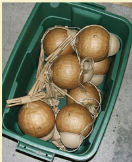
Figure 18: Finished shells utilizing vacu-form hemispheres. Note the vacu-form lift cups.
