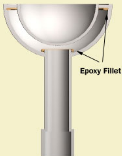
Figure 7: Attachment of mold components.
