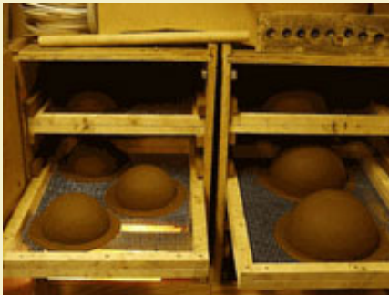
Figure 14: Assorted hemis drying in a dehumidified dry-box with circulated air.
