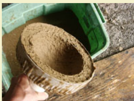
Figure 10: Removing loaded mold from tank.
