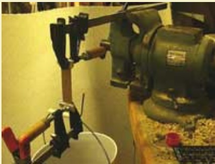
Figure 2: Another view of the bar clamps, held in place with a bench vise.
