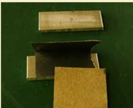
Figure 3: Aluminum plates and emery cloth used to evenly clamp the ends of paper strips.
