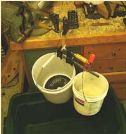
Figure 1: Bar clamps used in tensile strength measurement device.
