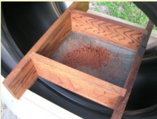
Figure 5: Pushing damp composition through the screen and into the spinning tire.
