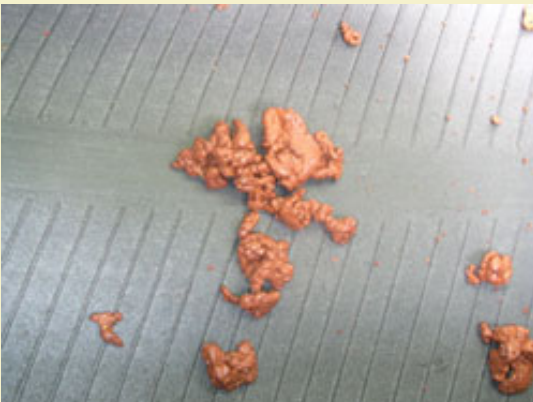
Figure 4: Clumped up mess resulting from over wetted composition (15% water).
