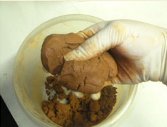
Figure 3: Over wetted composition with a clay like consistency will not work.
