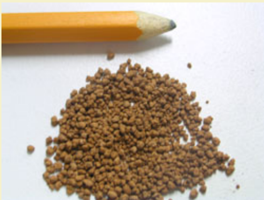
Figure 8: 31% passed through a 15 mesh screen.
