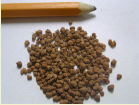
Figure 9: 55% passed through 8 mesh and sat on 15 mesh.
