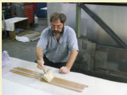
Figure 14: Applying paste to stacks of full-length strips.
