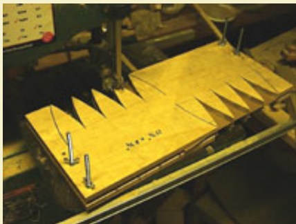
Figure 10: Cutting patterns on 100 sheets at once with a band saw jig.
