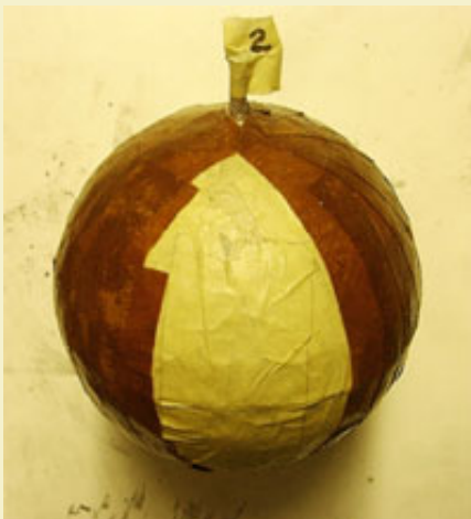
Figure 5: Working the pattern around the shell.
