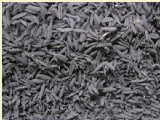
Figure 4: Closeup shows clean, unclumped hulls that flow easily even when wet.
