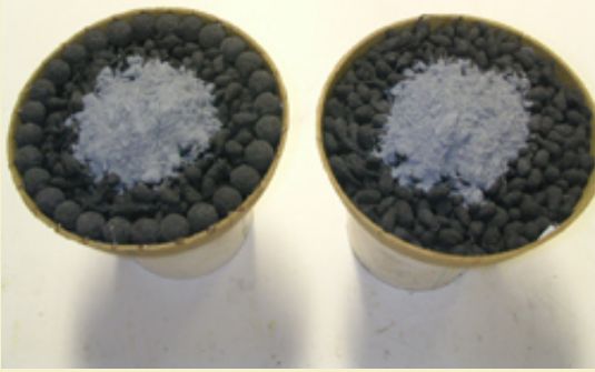
Figure 3: Flash booster poured loosely into the shell after loading.
