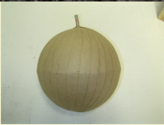
Figure 9: First layer after rolling out the wrinkles.
