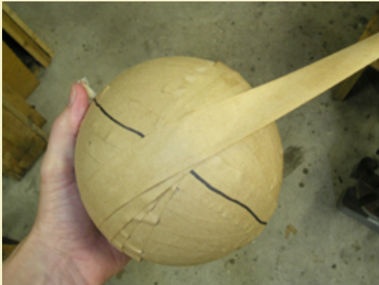
Figure 10: Starting the second layer, using a reference line to help locate the proper poles.
