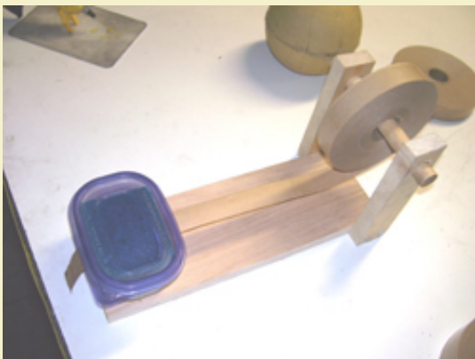
Figure 2: A simple tape dispenser that wets the gum as it is dispensed.
