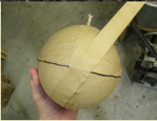
Figure 12: Starting the third layer, using another reference line to help keep the strips in the proper pattern.
