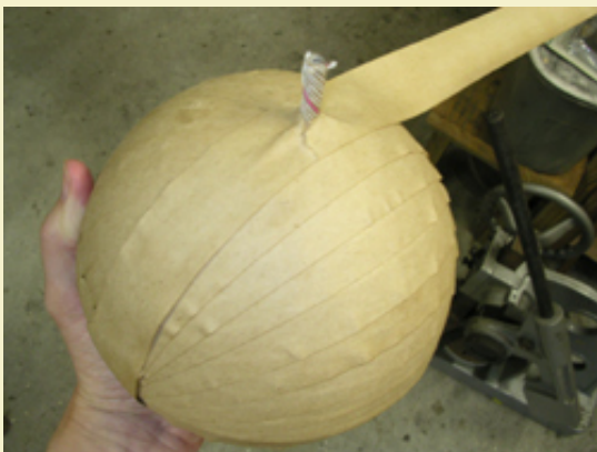
Figure 11: Tearing the strip to work around the time fuse.
