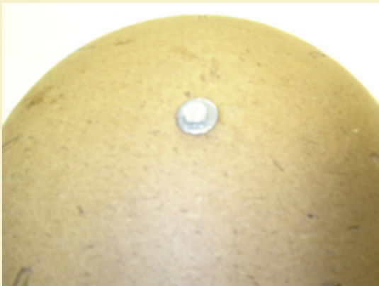
Figure 14: Plugging time fuse hole with a temporary nail before taping an 8" shell.
